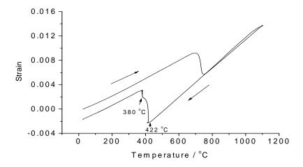
Fig. 5.7: Dilatometric curve designed for isotheral transformation at 380  $^\circ\!\mathrm{C}$
