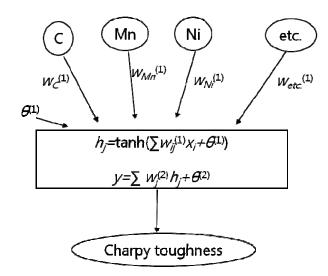
Fig. 1.3: Schematic illustration of the structure of a neural network
