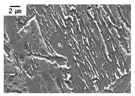
Fig. 5.8: Coalesced bainite in a sample designed for isothermal transformation at 380  $^{\circ}$ C in the 0.5Mn alloy. However, some transformation preceded the set temperature.
