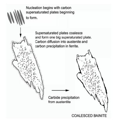
Fig. 1.8: Schematic diagram of the formation of coalesced bainite (Keehan, 2005)
