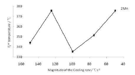
Fig. 3.3: Variation of  $T_S^{\gamma \alpha}$  of the 2Mn alloy with the magnitude of the cooling rate.
