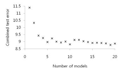
Fig. 4.2: The evolution of combined test error that was minimized with 19 sub-models.
