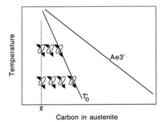
Fig. 5.1: Schematic diagram illustrating the degree of bainite transformation as temperature decreases.  $\overline{\mathbf{X}}$  is the average carbon concentration of the state,  $\mathbf{T'}_0$  is the  $\mathbf{T}_0$  curve adjusted for the stored energy of bainite and  $\mathbf{A}_{e3'}$  is the  $\alpha + \gamma / \gamma$  paraequilibrium phase boundary (Bhadeshia, 2001).
