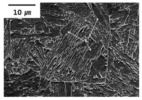
Fig. 5.11: Coalesced bainite in a sample transformed isothermally at 400  $^\circ\!C$  in the 0.5Mn alloy.
