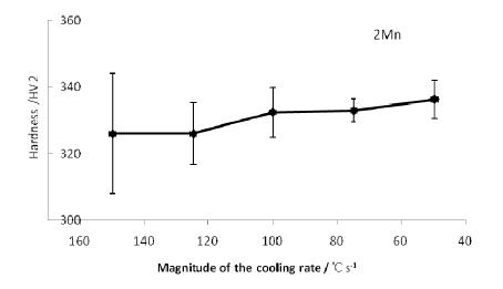
Fig. 3.4: Variation of hardness of the 2Mn alloy with the magnitude of the cooling rate
