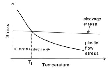
Fig. 1.2: Influence of temperature on the stress required for cleavage and plastic flow (Bhadeshia, 2001)
