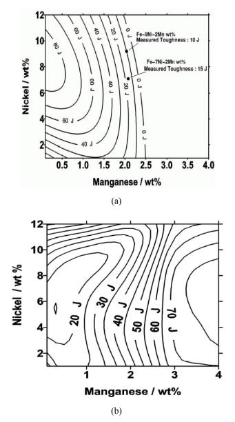
Fig. 1.7: Effect of manganese and nickel on toughness, as predicted using the neural network models (a) predictions (b)  $\pm 1\sigma$  uncertainty in prediction (Muruganath, 2002).
