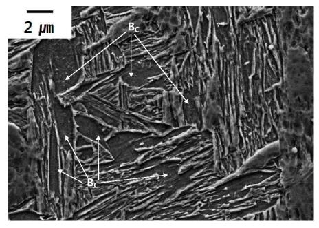
Fig. 5.10: Coalesced bainite in a sample designed for isothermal transformation at 390  $^\circ\!\!C$  in the 0.5Mn alloy.
