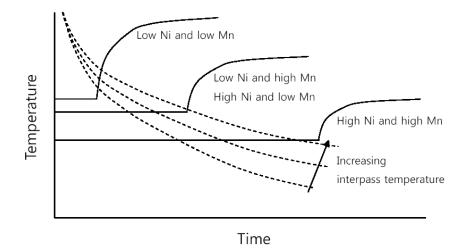
Fig. 4.15: Schematic diagram illustrating the effect of alloying solutes and interpass temperature on transformation temperature.
