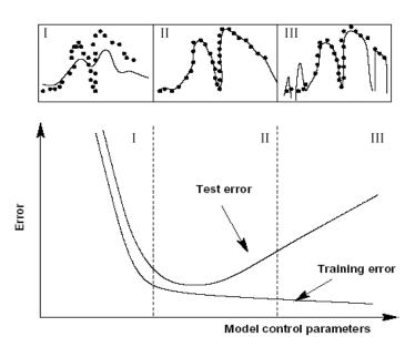
Fig. 1.5: Schematic diagram explaining the optimization of model complexity (MacKay, 1995a)
