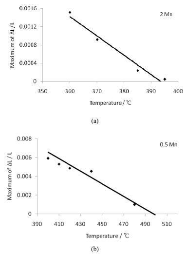
Fig. 5.3: Estimation of  $B_S$  of each alloy (a) the 2Mn alloy (b) the 0.5Mn alloy.  $\Delta L/L$  is the measured transformation strain.
