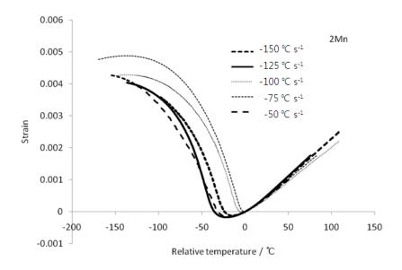
Fig. 3.9: Relative temperature- strain curves for the 2Mn alloy. At the origin, they have  $T_S^{\gamma \alpha}$  temperatures.
