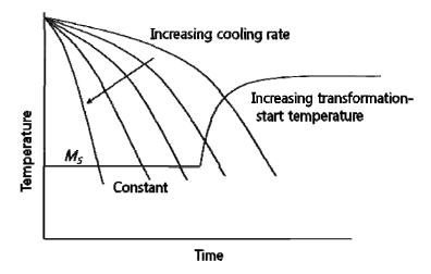
Fig. 3.1: Schematic diagram showing that  $M_{\rm S}$  corresponds the point at which  $T_{\rm S}^{\gamma\alpha}$  ceases to change as the cooling rate is increased.
