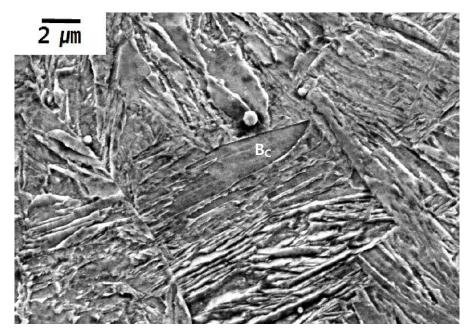
Fig. 5.6: Coalesced bainite formed by incomplete isothermal transformation at 370  $\,\,^\circ\!\mathrm{C}$  in the 2Mn alloy
