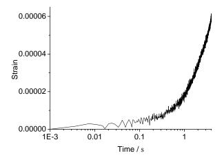
Fig. 5.5: Incomplete length change curve by isothermal transformation at 370  $\,^\circ\!\!{\rm C}$
