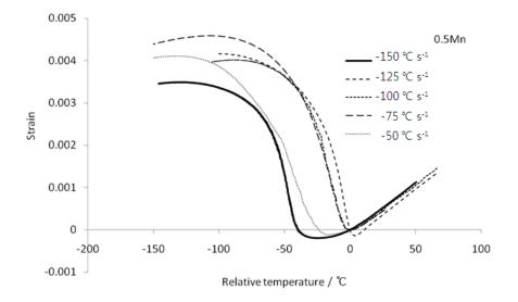
Fig. 3.10: Relative temperature-strain curves for the 0.5Mn alloy. At the origin, they have  $T_S^{\gamma\alpha}$  temperatures.
