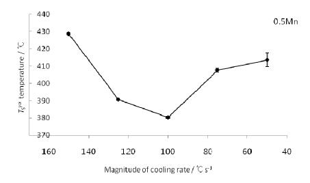
Fig. 3.7: Variation of  $T_S^{\gamma \alpha}$  of the 0.5Mn alloy with the magnitude of the cooling rate.
