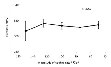
Fig. 3.8: Variation of hardness of the 0.5Mn alloy with the magnitude of the cooling rate
