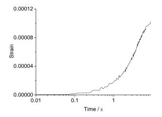
Fig. 5.9: Incomplete length change curve by isothermal transformation at 390  $^\circ$ C.
