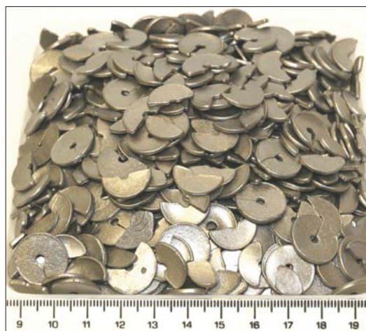
Two kilogrammes of titanium produced by Metalysis Ltd using a novel extraction process – the FFC Cambridge process
