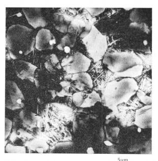
5 Alloy C after air cooling from the  $\alpha+\beta$  range; thin-foil electron micrograph  $\times 6\,000$
