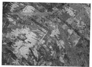
10 Specimen of U=0.5%Cr partially transformed at 450°C; polarized light  $\times\,150$
