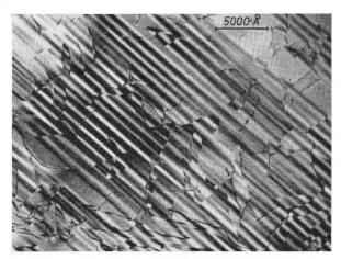
I Massive α-phase formed in a Cu-23·7 at-%Ga alloy on quenching from 780°C to room temperature; internal stacking faults inclined to the foil normal
