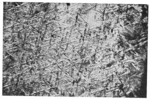
II Surface relief produced by partial transformation at 450°C; U-0.85% Cr  $\times$  150
