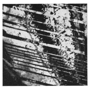
L Internally twinned martensite plates in 5wt-%Nb alloy
