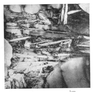
8 Alloy C after air cooling from the  $\alpha+\beta$  range; thin-foil electron micrograph  $\times 30~000$
