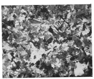
9 α-uranium in U-0·5%Cr formed by isothermal transformation at 450°C; polarized light ×150
