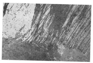
4 Transformation of a U-0.5% Cr alloy at 211°C showing one principal growth direction; polarized light ×150
