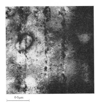
12 Alloy G after quenching from the  $\beta$  range and tempering at 550°C; thin-foil electron micrograph  $\times 40\,000$
