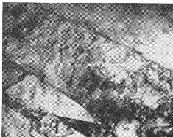
G 0.1% C, upper bainite formed at 450°C × 100000
