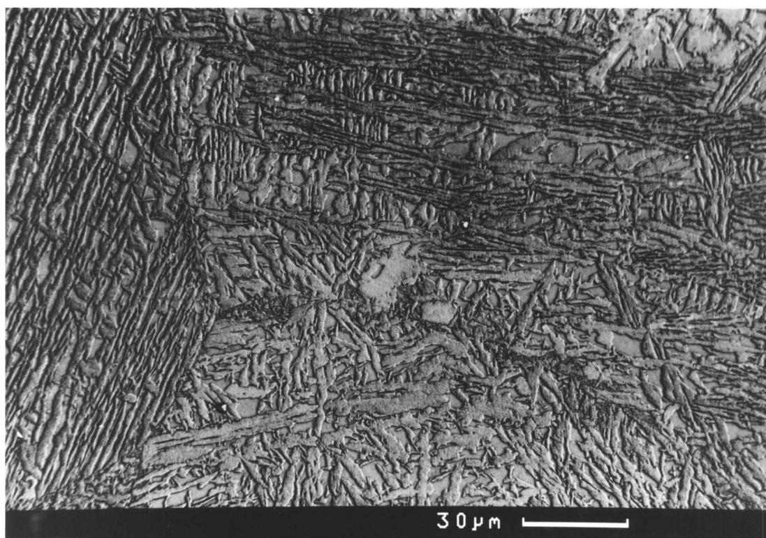
Figure 7.4 The microstructure of Alloy 5763 after austenitisation at  $1300^{\circ}\text{C}$  for 3 minutes followed isothermal transformation at  $500^{\circ}\text{C}$  to room temperature.
