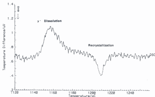
Fig. 2—Typical differential calorimetric curve illustrating the \gamma' is dissolution and recrystallization peaks. The heating rate is 10 K min -1 , the sample is from the intermediate region of the extruded bar, and the reference is a recrystallized sample of slightly smaller mass.
