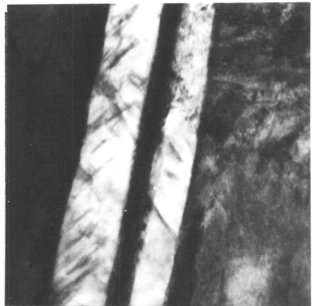
Figure I.13d Individual spikes of lower bainite after isothermal transformation at 257°C for 5 min.
