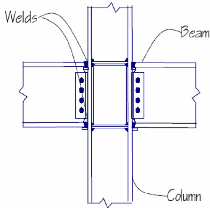
**The typical connection used prior to 1994. Severe stress concentrations inherent in its configuration were not considered in the design.**
