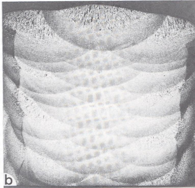
In multi-run welding, the temperature maintained immediately before depositing more metal
