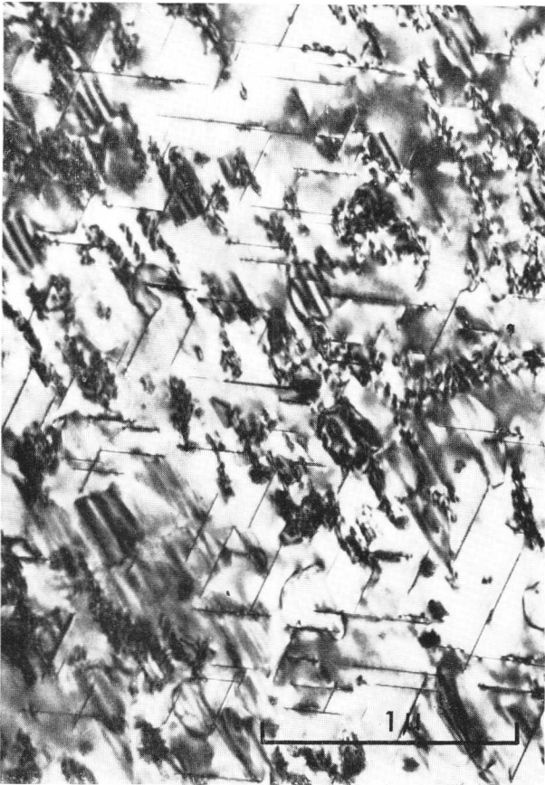
Fig. 1 Electron micrograph of the Al-2.5% Cu-0.5% Mg-0.5% Ag alloy aged at 225°C for 2 days; [110] zone axis showing two sets of plates edge on.
