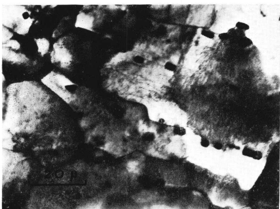
Fig. 2 Thin-foil micrograph of 0.21% plain carbon steel recrystallized as in Fig. 1(b), then creep-deformed 11% at 10,500 lb/in 2 and 700° C.
