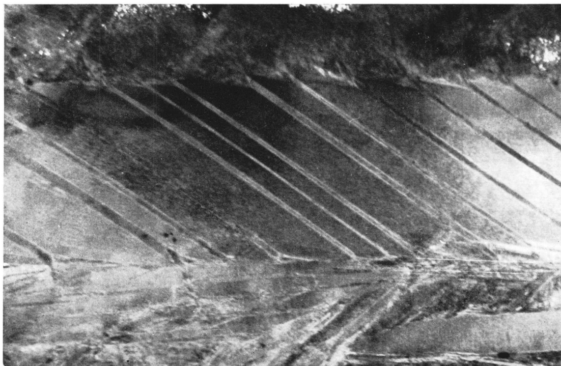
Fig. 2 Dark-field electron micrograph of a Ti-5% Mn alloy, water-quenched from 850°C and aged at 400°C for 2 h. 80 The \alpha (hexagonal) plate is twinned on \{10\bar{1}1\}_\alpha and is in a \beta matrix. The habit plane of the plate is \sim\{344\}_\beta but the individual interfaces of the two twin orientations are \sim\{334\}_\beta . \times 20,000 .
