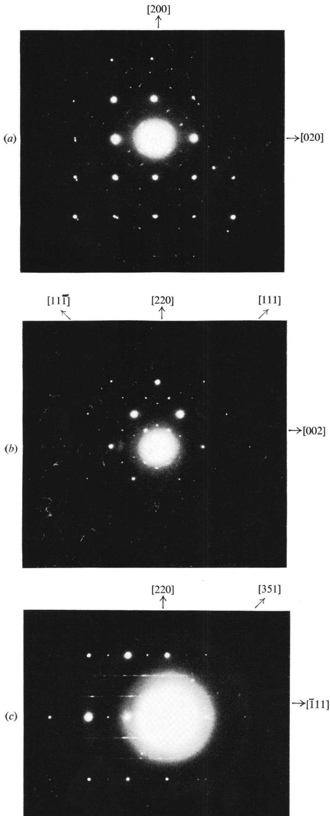
Fig. D.V.2. Electron-diffraction patterns of  $M_4C_3$ : (a) [001] zone, (b) [110] zone, and (c) [112] zone. (Dyson and Andrews.)
