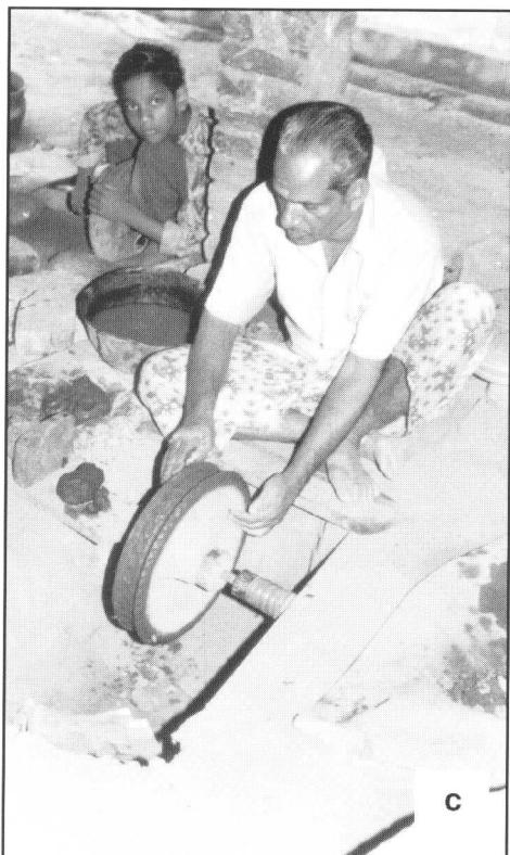
Fig. 21 : (c) Applying a layer of fine powder mix followed by wax layer required to achieve the thickness of the vessel
