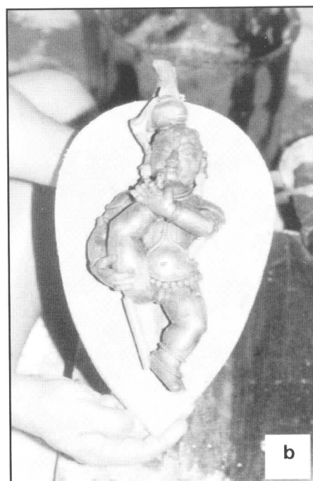
Fig. 15 : a) Completed individual wax model/pattern of child Krishna and banyan tree leaf (b). Completed wax pattern of child Krishna on that of banyan tree leaf.
