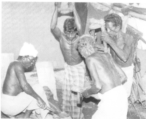
Fig. 5 : Rhythmic hammering of the disks into a bowl shape by three men as the chief craftsman controls the progress.
