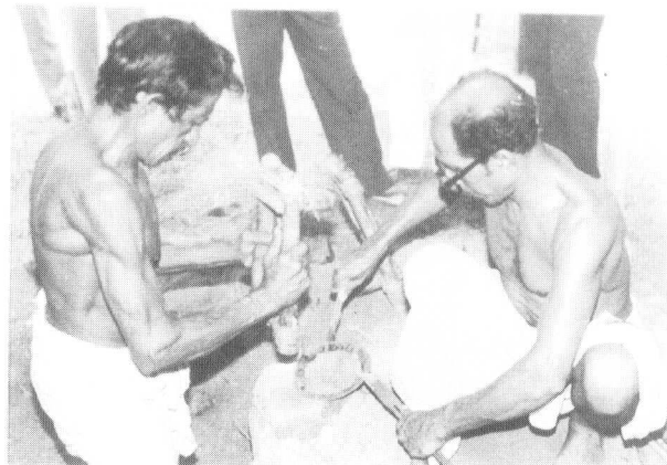
Fig. 6 : Continuation of working after reheating, which are continued until the desired shape is achieved
