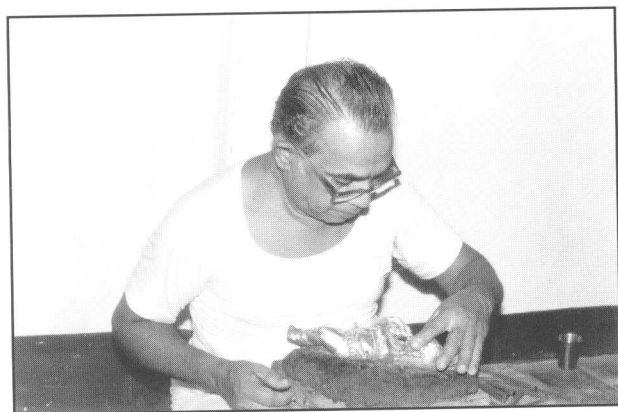
Fig. 19 : Fixing child Krishna casting on wax bed spread over a wooden plate for finishing operation.
