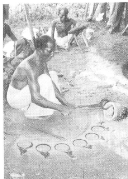
Fig. 4 : Casting of high tin bronze disks in open sand moulds.
