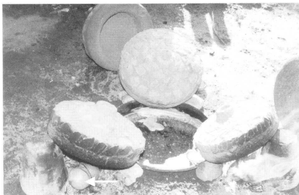
Fig. 22 : Dewaxing by heating the moulds by coconut shells (shown by arrow) in progress and collection of molten wax in vessel for three moulds.
