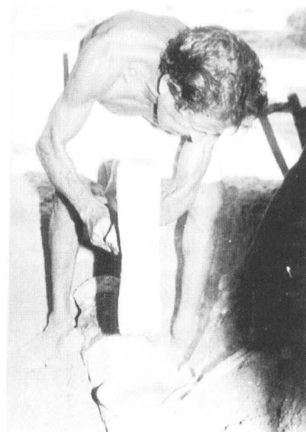
Fig. 7 : Conducting the last phase of the hot working operation with a wooden log and a wooden mallet prior to heating again and quenching in water.
