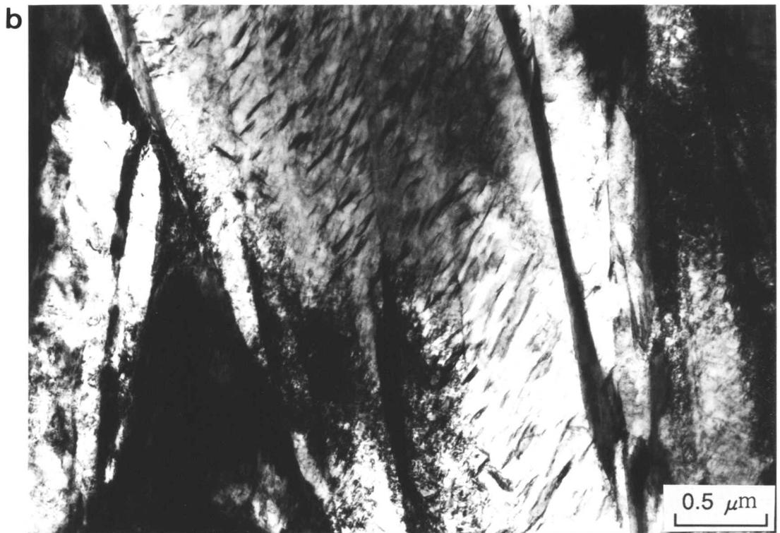
Fig. 4.12 Typical TEM micrographs of upper and lower bainite obtained in the Fe-0.43C-2.0Si-3.0Mn alloy at a) 350 °C and b) 270 °C respectively.
