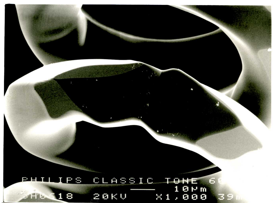
Micrograph 6 Philips Classic tone 60W, Matched facets, mirrored in grain boundary. Increased evaporation from grain boundary.
