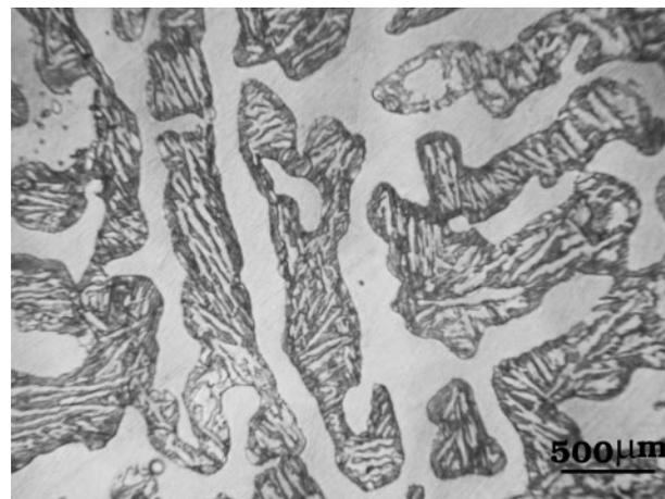
7 The microstructure of  $\delta$ -TRIP steel<sup>76</sup>
