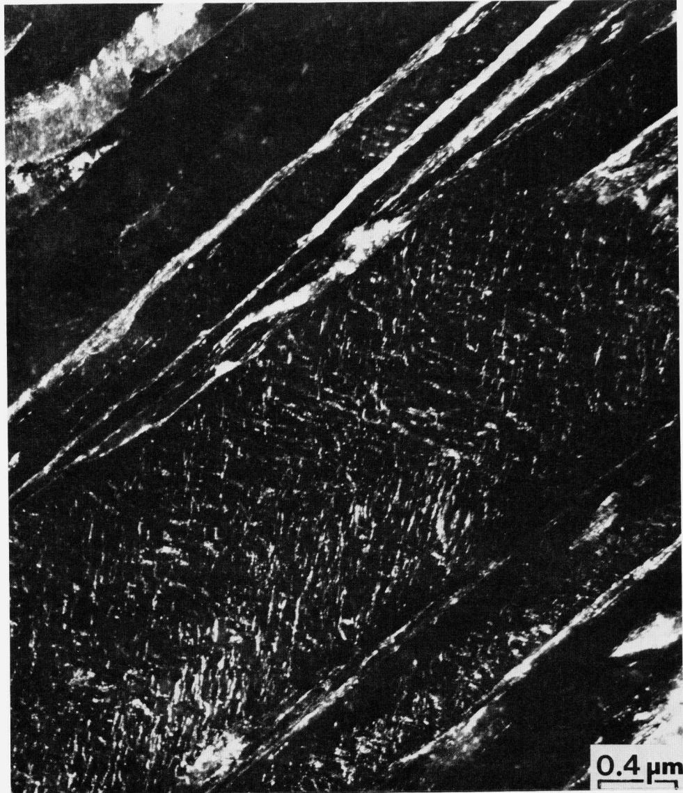
Figure 11. Fine structure of 4130 steel tempered at 150°C. Darkfield transmission electron micrograph. Courtesy of M. Losz.
