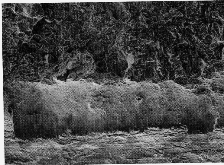
Figure 5. Top view of shear initiation zone in 4340 steel tempered at 200°C. Notch is at bottom. SEM micrograph (18).
