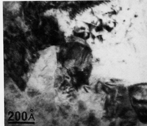
Fig. 10a. Bright field transmission electron micrograph showing a La-P-O precipitate in RSP Ni-Mo steel.
