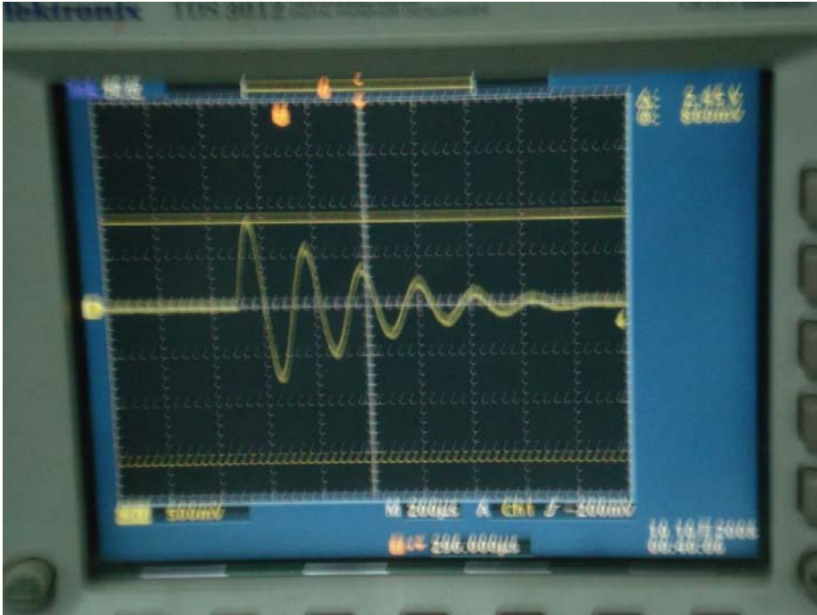
Fig. 3.6: Electropulsing waveform as observed in the oscilloscope
