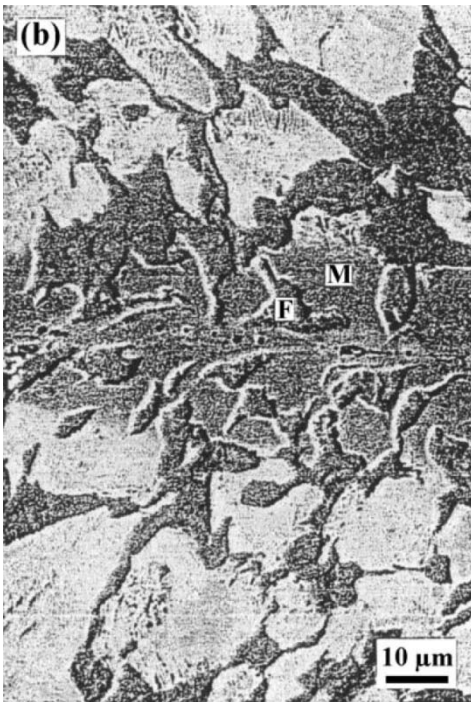
Fig. 1.5: a) Optical b) SEM micro graph of a crack partially healed by electropulsing (F=ferrite M=martensite) [Zhou et al. , 2004]
