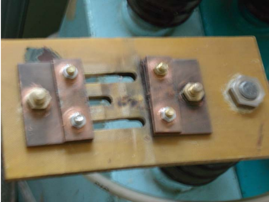
Fig. 3.3: The large copper electrode cum heat sink used for electropulsing the steel samples
