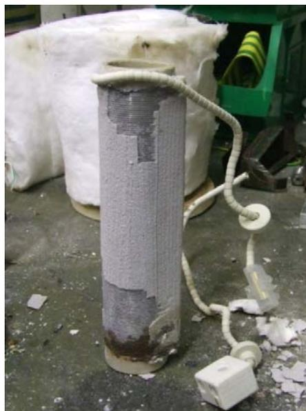
**Figure 5-66: the damage occurred to the furnace after using brine solution as a quenchant.**
