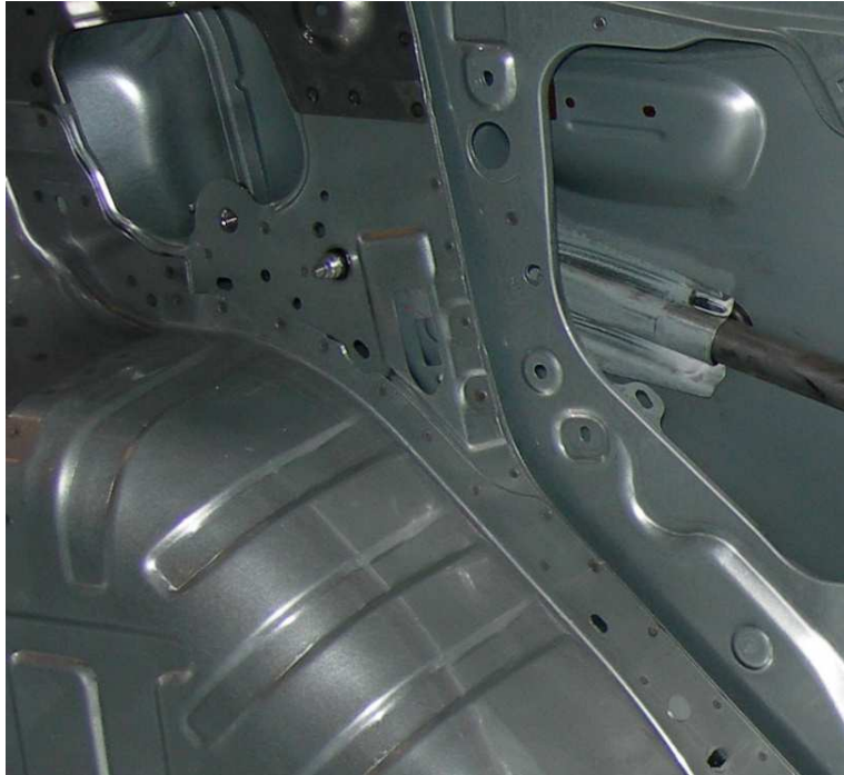
Figure 2: An illustration of some of the spot welds providing integrity to the body of a car.
