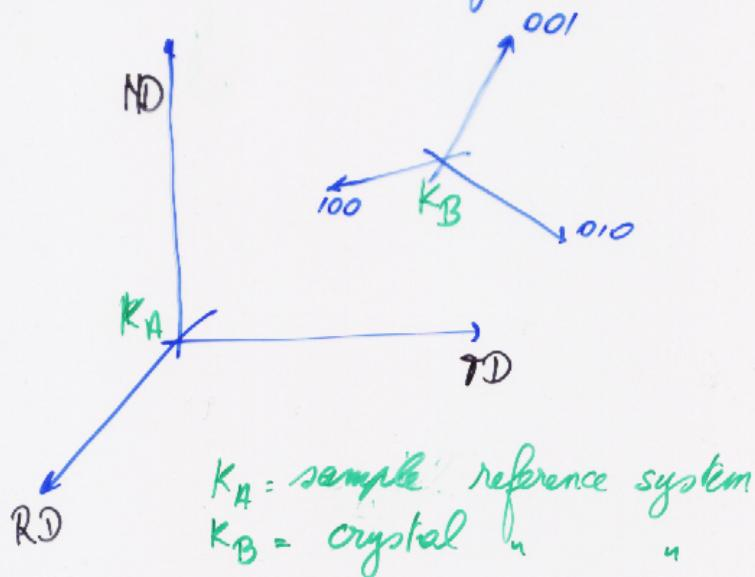
Suppose  $a_{ij}$  = direction cosine of sample axis  $x_j$  with respect to crystal axis  $x'_i$ :
