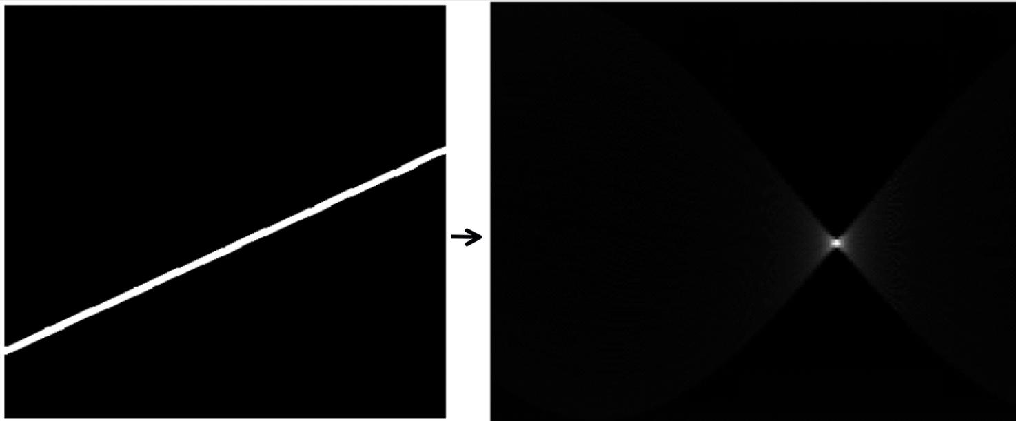
thus, straight lines in the original image (i.e. bands) can be identified by detecting the local maxima in Hough space
