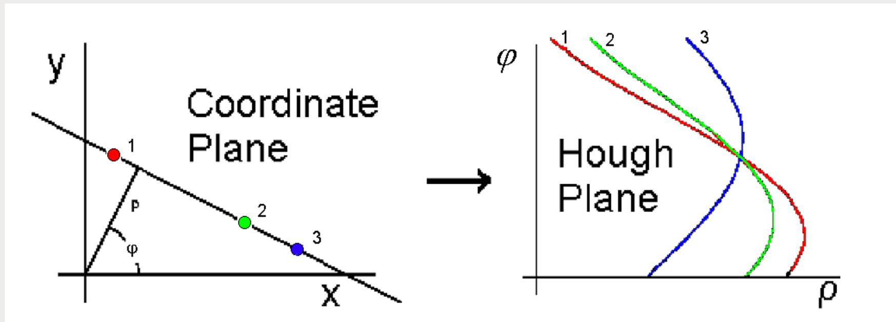
objective: convert the parallel lines / bands found in EBSD patterns into points. These points can more easily be identified and used in automatic computation.
