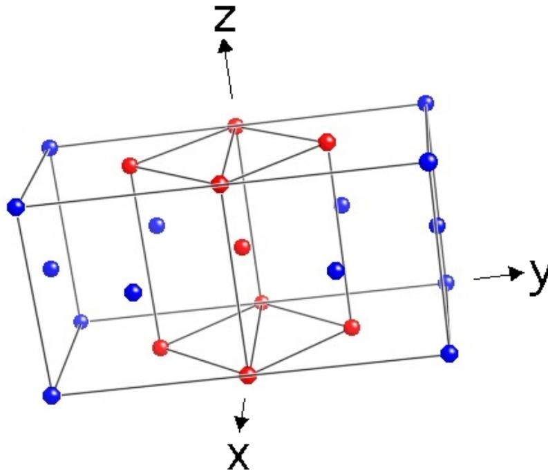
Figure 2: Two face-centred cubic unit cells of austenite, together with a body-centred tetragonal cell of austenite. The Bain strain (not illustrated here) involves a compression of the body--centred tetragonal cell of austenite along  $z$  and a uniform expansion on the  $x$ - $y$  plane.
