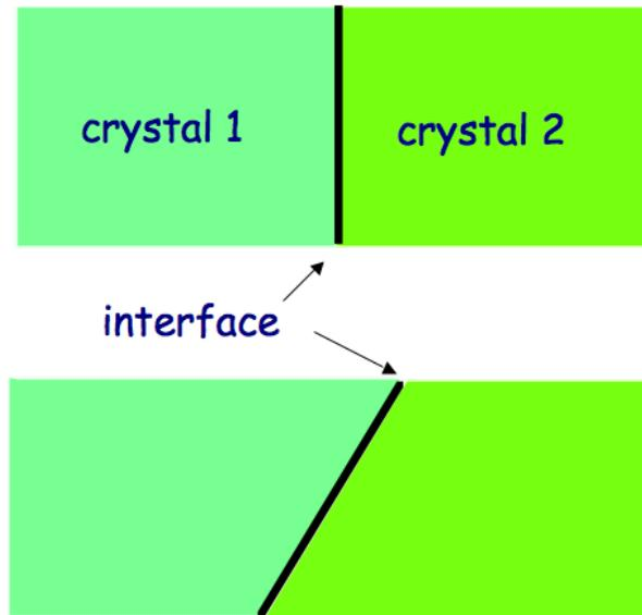
Fig. 5: The conventional degrees of freedom associated with a bicrystal containing an interface. Translations in the plane of the interface are neglected here.
