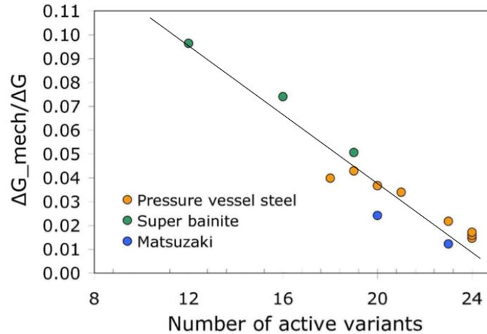
Figure 8: The ratio of the mechanical to total driving force for transformation as a function of the number of active variants for a variety of steels [25].
