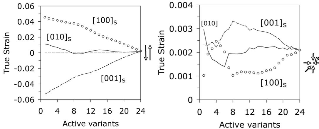
Fig. 7: (a) Transformation strain along the sample axes when a polycrystalline sample is subjected to pure shear; (b) much small strains when subjected to hydrostatic compression. After Kundu et al. [25].
