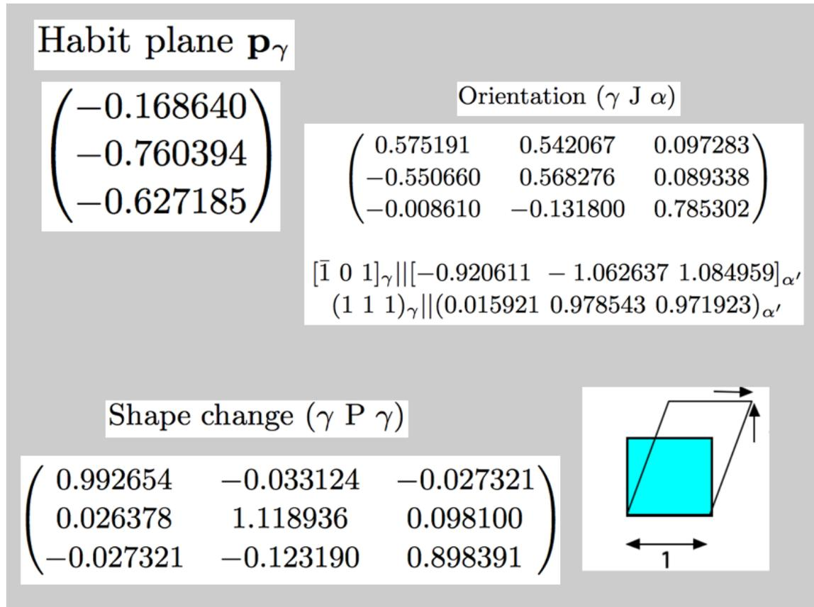
Fig. 6: An example of a complete crystallographic set describing a single plate of martensite, including the habit plane, the shape deformation and the orientation relationship (and implicitly the lattice-invariant deformation). All of these quantities are mathematically connected and cannot in general be varied independently.
