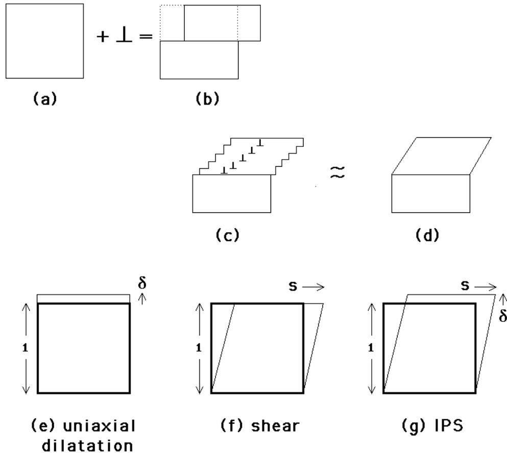
Fig. 1 (a, b) Step caused by the passage of a slip dislocation. (c, d) Many slip dislocations, causing a macroscopic shear. (e) An invariant-plane strain with a uniaxial dilatation. (f) An invariant-plane strain which is a simple shear. (g) An invariant-plane strain which is the combined effect of a uniaxial dilatation and a simple shear.
