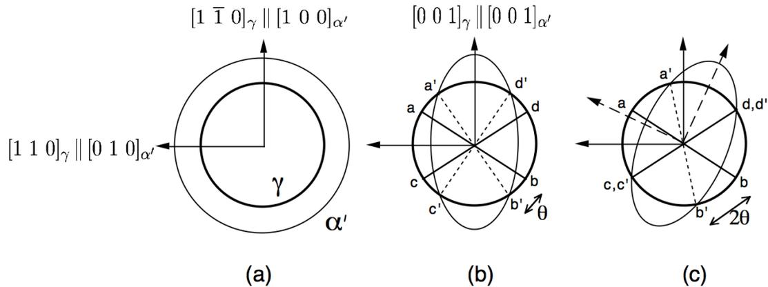
Fig. 3: (a) and (b) show the effect of the Bain strain on austenite, which when undeformed is represented as a sphere in three-dimensions. The strain transforms it to an ellipsoid of revolution. (c) shows the ILS obtained by combining the Bain strain with a rigid body rotation through an angle  $\theta$ .
