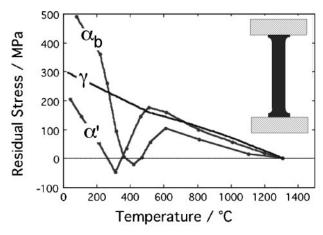
1 Development of stress as tensile test sample which is austenitic at high temperatures is constrained (inset) and then allowed to  $cool:^{19}$  sample labelled  $\gamma$  remains austenitic ( $\gamma$ ) at all temperatures, whereas other two transform either into bainite ( $\alpha$ <sub>b</sub>) or ( $\alpha$ ')
