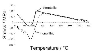
4 Satoh tests on martensitic weld alloy<sup>15</sup> using bimetallic sample, and one manufactured entirely from test alloy
