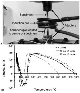
2 a Satoh test in progress: gradient of colour along length of sample is due to variations in temperature; these gradients compromise relationship between recorded stress and temperature, and b variations along length of sample
