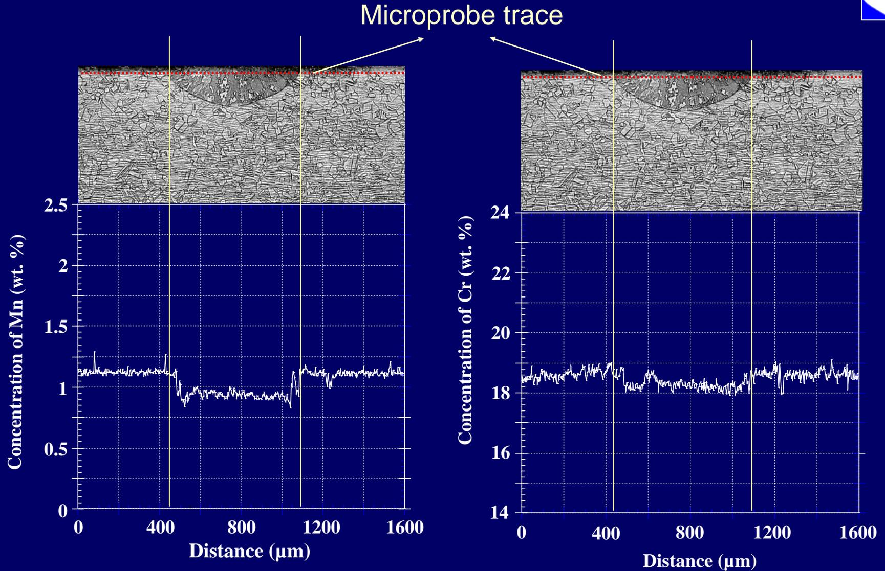
Laser power: 1067 W, pulse duration: 3.0 ms, and beam radius: 0.325 mm 48
