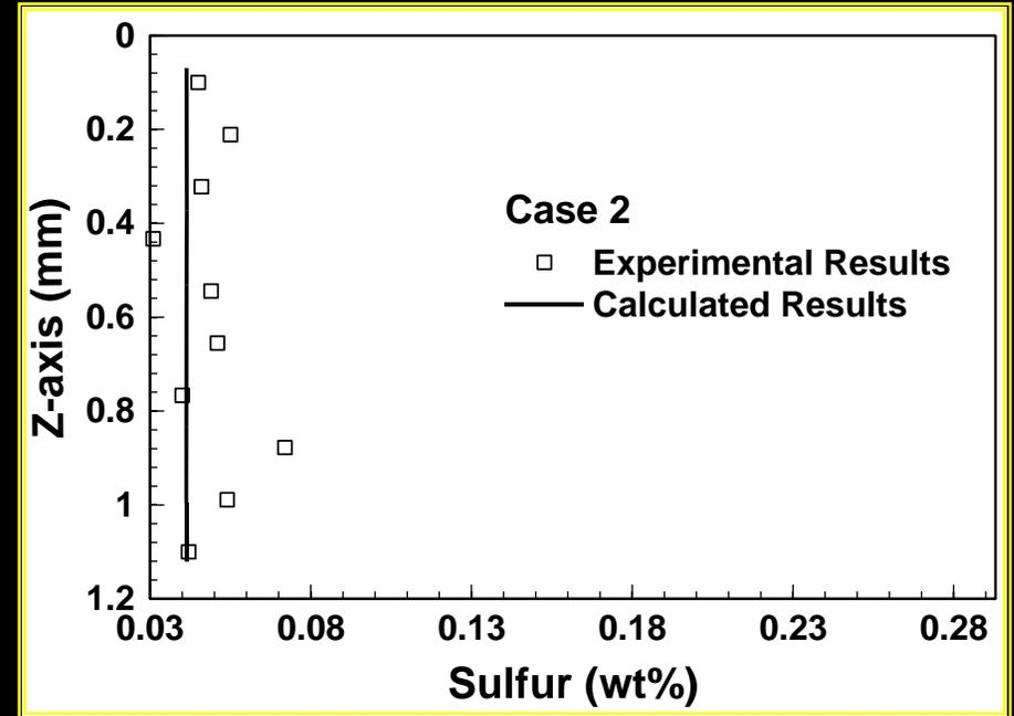
*Welding conditions: 150 A, 10.8 V, welding speed is 1.7 mm/s*
