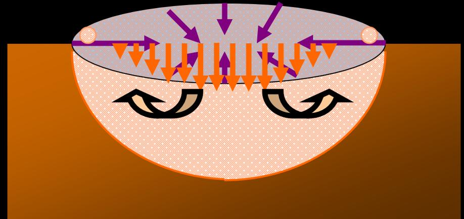
$t > 2.6$  ms, Recoil force  $>$  Surface tension force  $\Rightarrow$  Expulsion of metal drops
