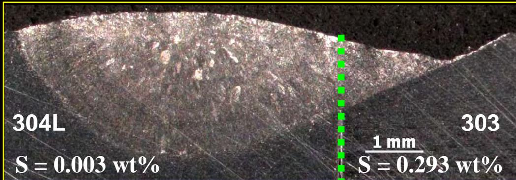
$I = 150 \text{ A}$ ,  $V = 10.5 \text{ V}$ , Welding speed =  $1.7 \text{ mm/s}$
