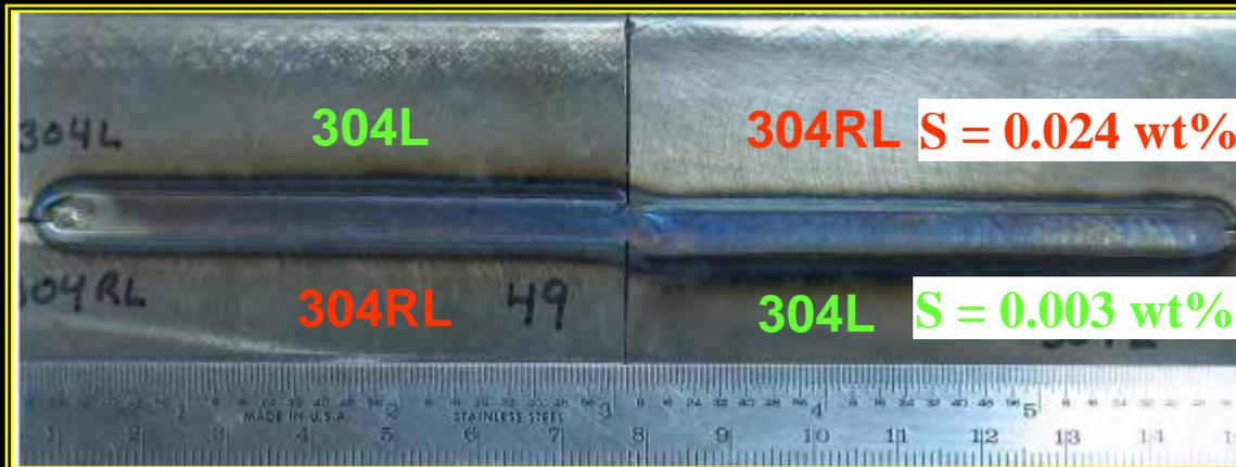
$I = 101 \text{ A}$ ,  $V = 9.6 \text{ V}$ , Welding speed =  $1.7 \text{ mm/s}$
