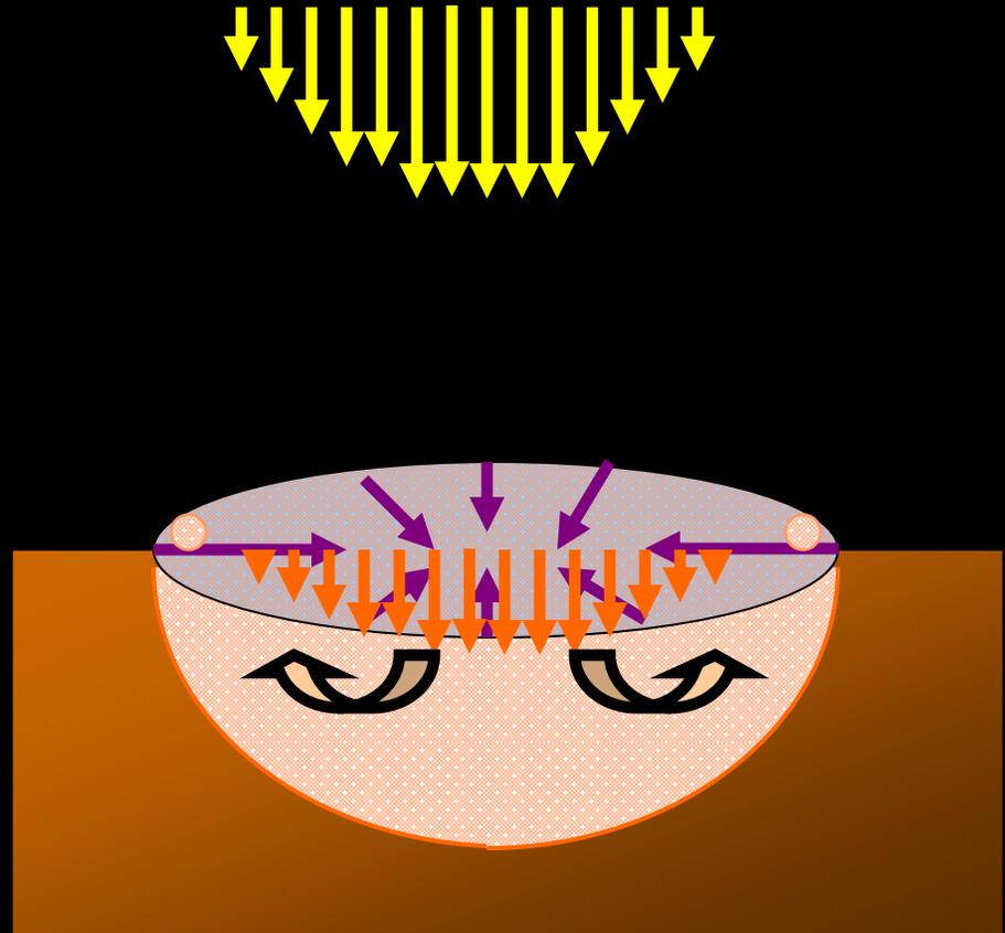
Surface tension force:  $F_s = 2\pi r_0 \sigma$
