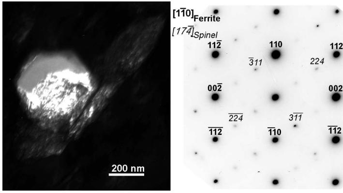
Figure 9: a) Dark field transmission electron micrograph of an inclusion and an adjacent ferrite grain. b) The corresponding selected area electron diffraction pattern with indexed reflection for both the ferrite grain and the  $\text{MnTi}_2\text{O}_4$ –spinel phase of the inclusion. Extra reflections are due to double diffraction.
