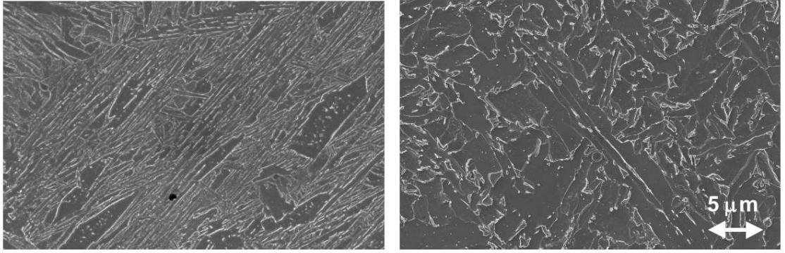
Figure 5: FEGSEM micrographs presenting an overview of the as-deposited last bead microstructure for two different cooling times. Lower bainite, martensite and coalesced bainite are the main constituents in the rapidly cooled weld metal on the left, whereas the more slowly cooled structure consists largely of upper bainite.
