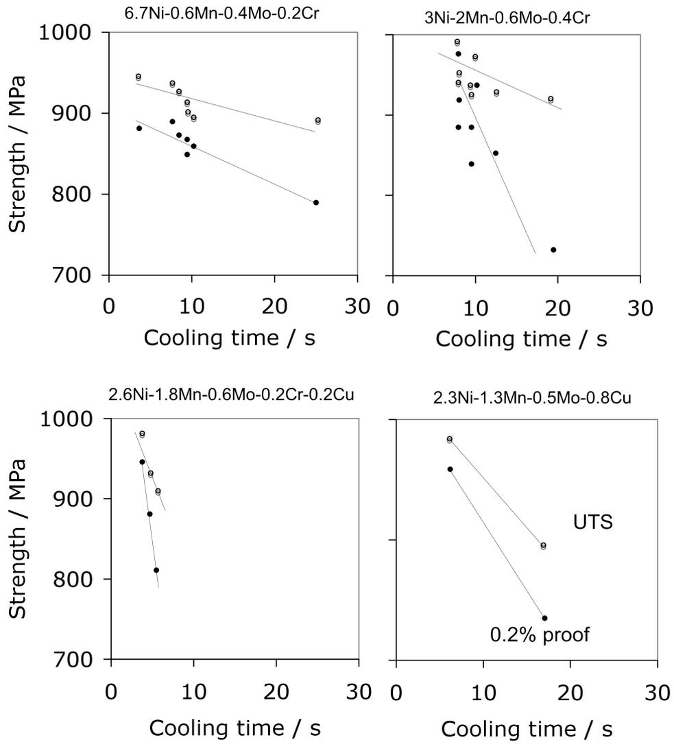
Figure 4: Strength as a function of cooling time between 800 and 500°C for weld metals with Ni contents in the range 2.3–6.7 wt%, [18].
