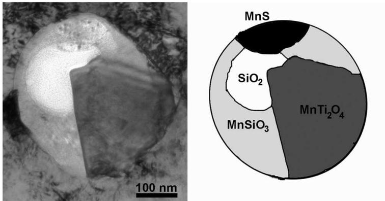
Figure 8: a) Bright field transmission electron micrograph of an inclusion. b) Schematic representation of the inclusion, showing the morphology of present phases.
