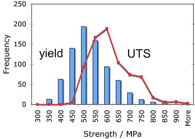
Figure 1: Distribution of strength in ferritic steel weld metals, incorporating data from some 800 welding alloys. UTS stands for the ultimate tensile strength. Data from [4].
