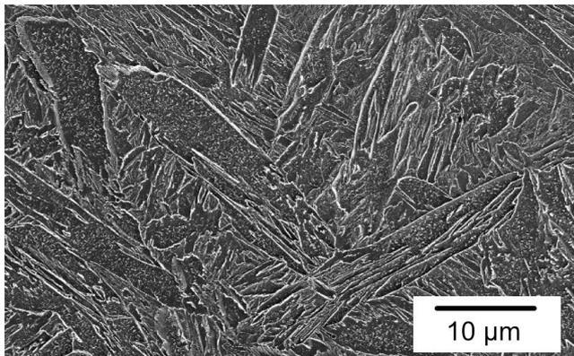
Figure 3: Large coalesced bainite grains in the last bead of a 0.08C–10Cr–1Ni–0.3Mo wt% high strength weld metal with 910 MPa in yield strength.
