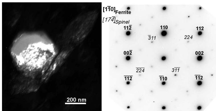
Figure 9: a) Dark field transmission electron micrograph of an inclusion and an adjacent ferrite grain. b) The corresponding selected area electron diffraction pattern with indexed reflection for both the ferrite grain and the  $\text{MnTi}_2\text{O}_4$ -spinel phase of the inclusion. Extra reflections are due to double diffraction.
