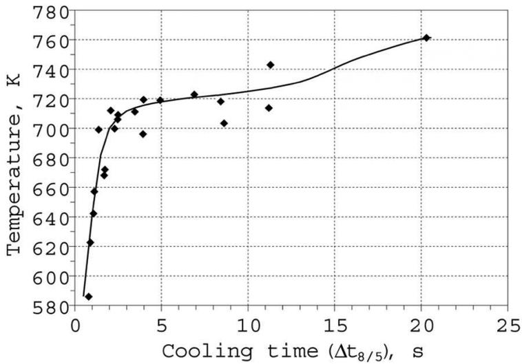
Figure 6: Experimental CCT-diagram for OK 75.78 displaying transformation start temperatures as a function of cooling time between 800C and 500C. Transformation temperatures gradually increase with cooling time above 3s and decrease rapidly for shorter cooling times.
