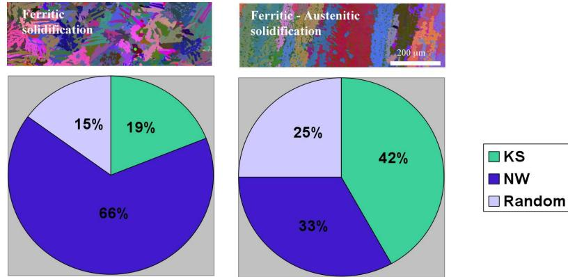
Figure 16: EBSD orientation maps (top) and classification of austenite/ferrite boundary orientations (below) for weld metals with a fully ferritic solidification (left) and mixed ferritic-austenitic solidification (right). More phase boundaries had a random orientation relationship after mixed mode solidification. The NW relationship was most frequent after fully ferritic solidification whereas KS was more common after a mixed mode solidification
