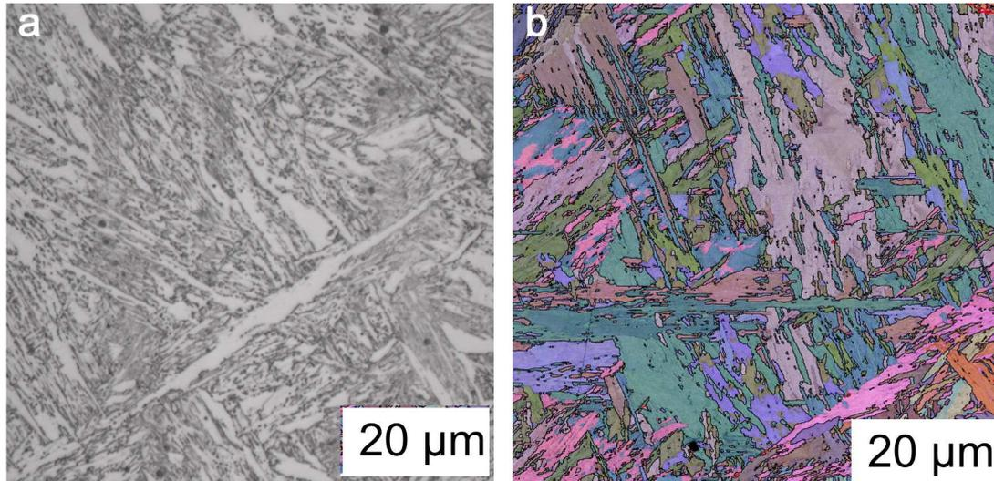
Figure 11: (a) LOM micrograph showing the etched microstructure of a 7Ni weld metal. (b) EBSD orientation map from the same microstructure.
