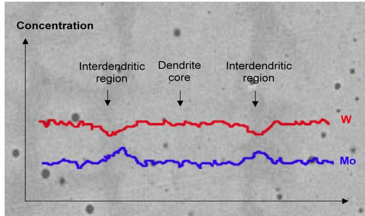
Figure 18: Concentration profiles for W and Mo across dendrites in a Ni-based weld metal. Mo is enriched in interdendritic regions whereas W is depleted resulting in a more even distribution of alloying elements and thereby better corrosion resistance. Dendrite spacing is approximately 10  $\mu\text{m}$ .
