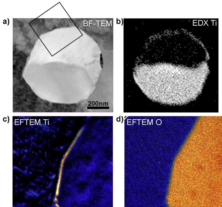
Figure 10: Bright field transmission electron micrograph of an inclusion. An EDX titanium map of the inclusion is shown in b). Energy filtered transmission electron micrographs of titanium and oxygen elemental maps are shown in c) and d), respectively. The maps were recorded over the area marked with a black square in a).
