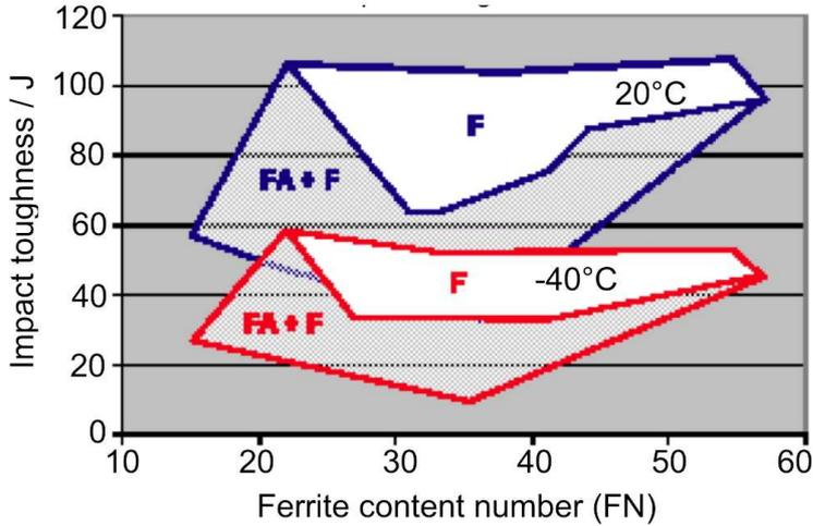
Figure 15: Impact toughness scatter bands for lean duplex weld metals with a fully ferritic solidification (F) and those with regions having a morphology with ferrite located mainly interdentritically and forming an almost continuous network typical of mixed austenitic-ferritic solidification (FA). The minimum values and scatter increase significantly with mixed mode solidification.
