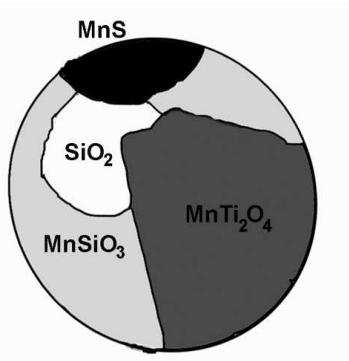
Figure 8: a) Bright field transmission electron micrograph of an inclusion. b) Schematic representation of the inclusion, showing the morphology of present phases.
