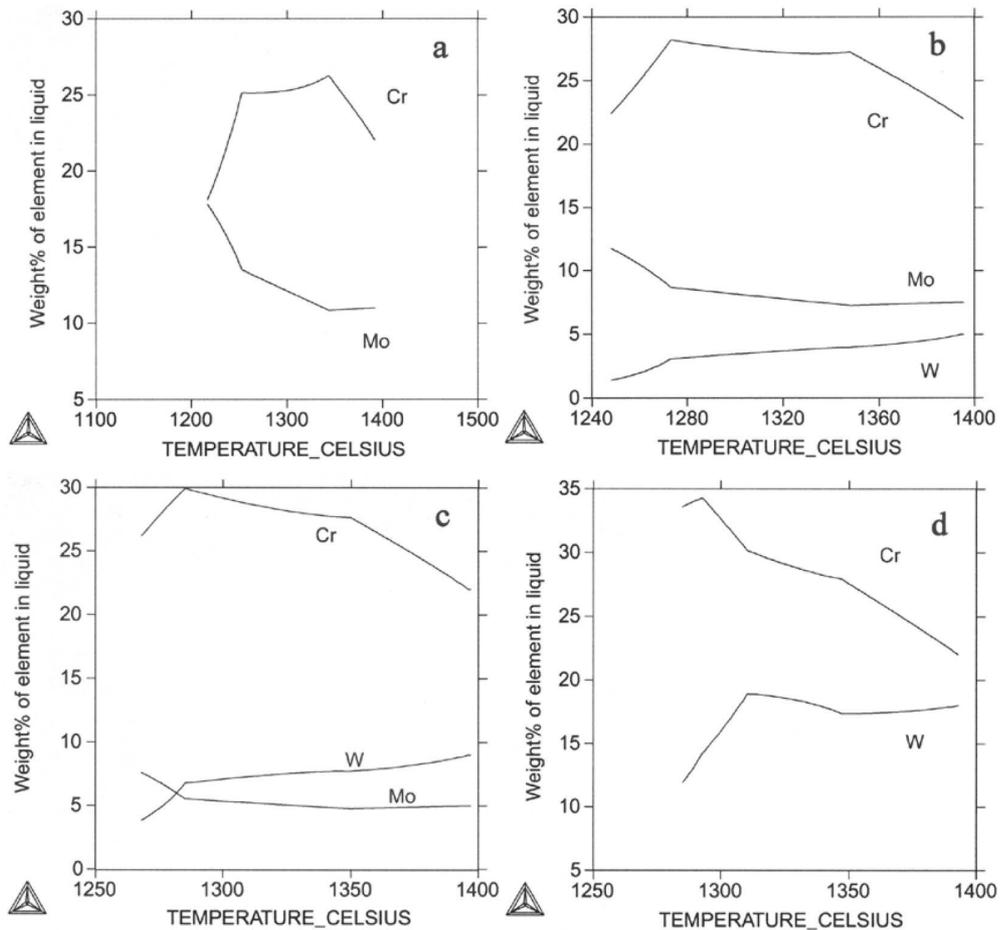
Figure 17: Thermo-Calc results from the Scheil calculations showing the concentration of elements in the liquid during solidification. At lower temperatures changes occur because of precipitation, which is probably too slow to take place in practise. The base composition was Ni - 0.05C, 0.5Si, 1Mn and 22Cr wt%, with varying amounts of Mo and W. a) 11Mo, b) 7.5Mo-5W, c) 5Mo-9W and d) 18W.
