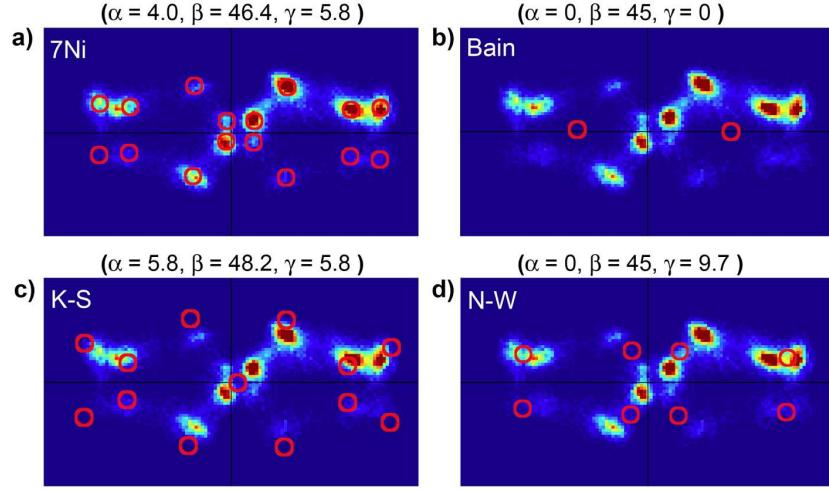
Figure 12: Bain zone from a  $\{111\}$  experimental pole figure, colour-coded with respect to intensity. Theoretical poles for the different ORs 7Ni (best fit), Bain, K-S and N-W are marked with red circles in a)-d), respectively. The Euler angles are also given for each OR.
