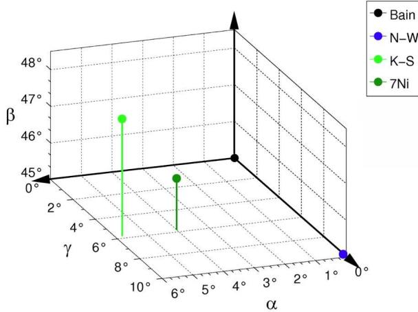
Figure 13: Euler space representation of the OR between austenite and ferrite in a 7Ni weld metal. Common rational ORs are also displayed for the purpose of reference.
