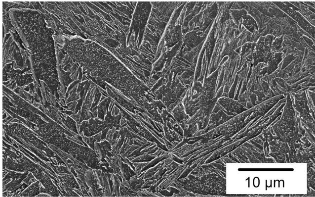
Figure 3: Large coalesced bainite grains in the last bead of a 0.08C–10Cr–1Ni–0.3Mo wt% high strength weld metal with 910 MPa in yield strength.
