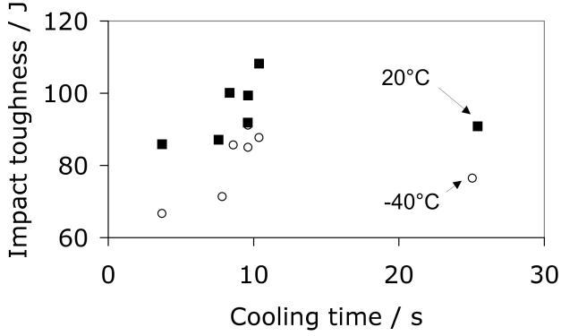
Figure 7: Impact toughness as a function of cooling time ( $\Delta t_{8/5}$ ) for a highly alloyed high strength weld metal.
