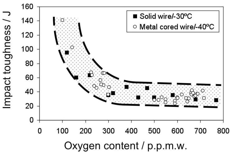
Figure 2: Effect of oxygen content on Charpy–V impact toughness of supermartensitic weld metals on. Weld metals produced with different welding processes and different consumables all fall within the same scatter band [6].
