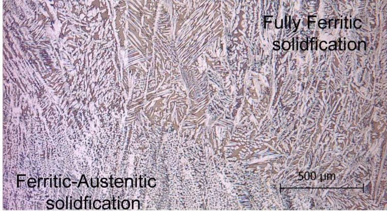
Figure 14: Lean duplex weld metal with regions of Widmanstätten-type austenite typical of a fully ferritic solidification (top) and regions having a morphology with ferrite located mainly interdendritically and forming an almost continuous network typical of mixed austenitic-ferritic solidification (bottom).
