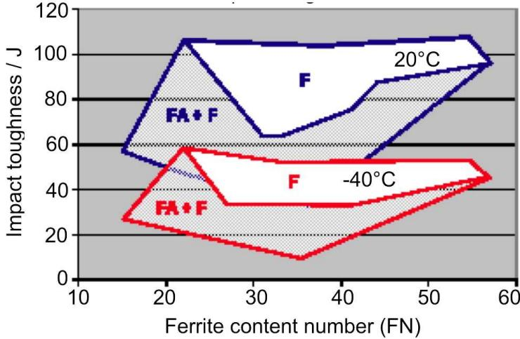
Figure 15: Impact toughness scatter bands for lean duplex weld metals with a fully ferritic solidification (F) and those with regions having a morphology with ferrite located mainly interden-dritically and forming an almost continuous network typical of mixed austenitic-ferritic solidification (FA). The minimum values and scatter increase significantly with mixed mode solidification.
