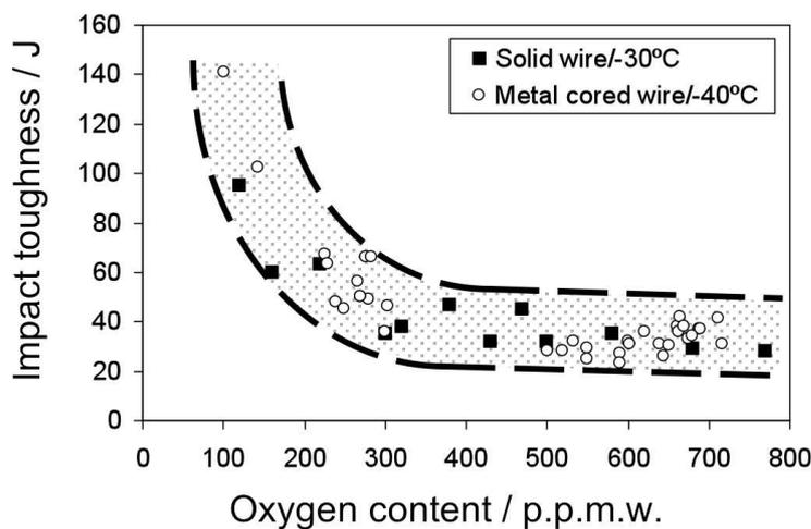
Figure 2: Effect of oxygen content on Charpy-V impact toughness of supermartensitic weld metals on. Weld metals produced with different welding processes and different consumables all fall within the same scatter band [6].
