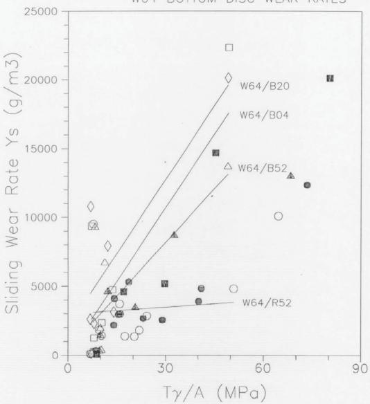
Figure 10.7 Sliding wear rate Y<sub>s</sub> plotted linearly against Tγ/A for bottom (driving) W64 discs except those run against top discs with mild wear rates (less than 200 g/m³).
