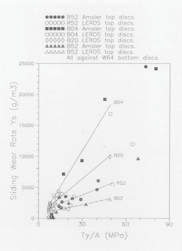
Figure 10.6 Sliding wear rate  $Y_s$  plotted linearly against  $T\gamma/A$  for top (driven, "braking") discs except those with mild wear rates (less than 200 g/m<sup>3</sup>).
