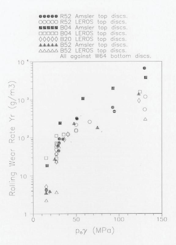
Figure 10.1 Rolling wear rate Y<sub>r</sub> plotted logarithmically against p<sub>o</sub>γ for all top (driven, "braking") discs tested.
