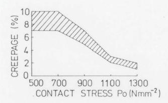
Figure 10.9 Transition zone, with respect to test conditions, from type I, "mild" wear to type II "severe" wear for standard BS11(0.53wt.%C) rail steel. From Bolton and Clayton's Amsler test results[Bolton & Clayton, 1984].
