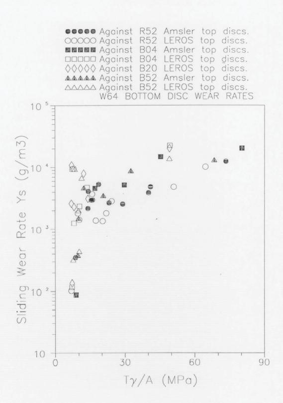
Figure 10.5 Sliding wear rate Y<sub>s</sub> plotted logarithmically against Tγ/A for all bottom (driving) W64 discs tested.
