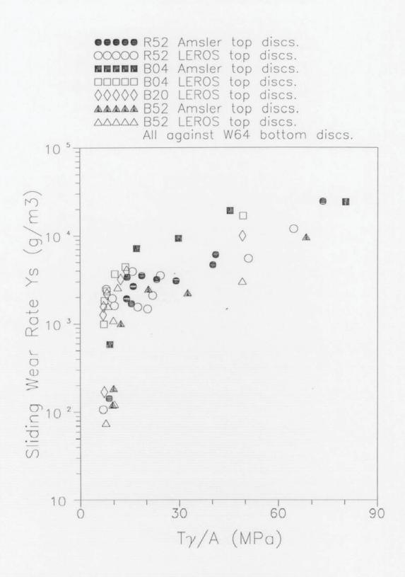
Figure 10.4 Sliding wear rate Y<sub>s</sub> plotted logarithmically against Tγ/A for all top (driven, "braking") discs tested.
