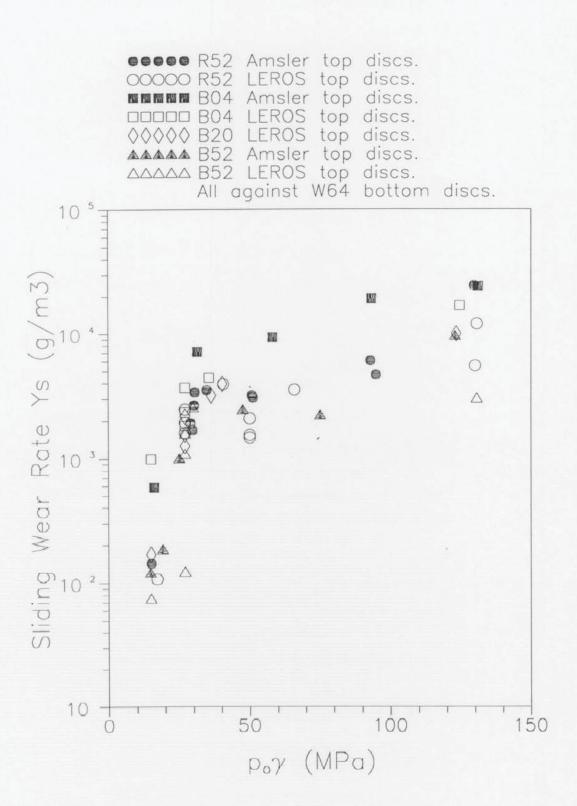
Figure 10.3 Sliding wear rate  $Y_s$  plotted logarithmically against  $p_o \gamma$  for all top (driven, "braking") discs tested.
