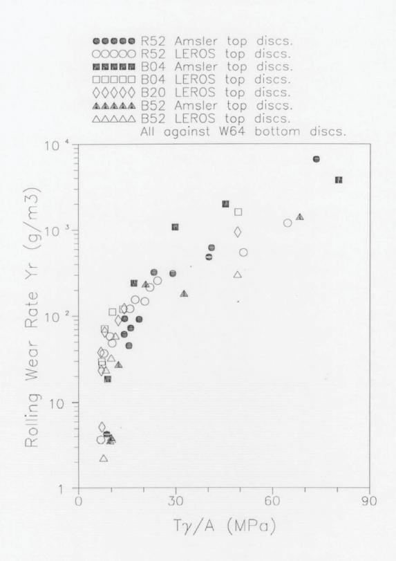
Figure 10.2 Rolling wear rate Y<sub>r</sub> plotted logarithmically against Tγ/A for all top (driven, "braking") discs tested.
