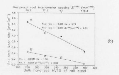
Figure 10.8 The relationship between pearlitic rail steel wear and interlamellar spacing for different types of wear test[from Perez & Beynon, 1993].
