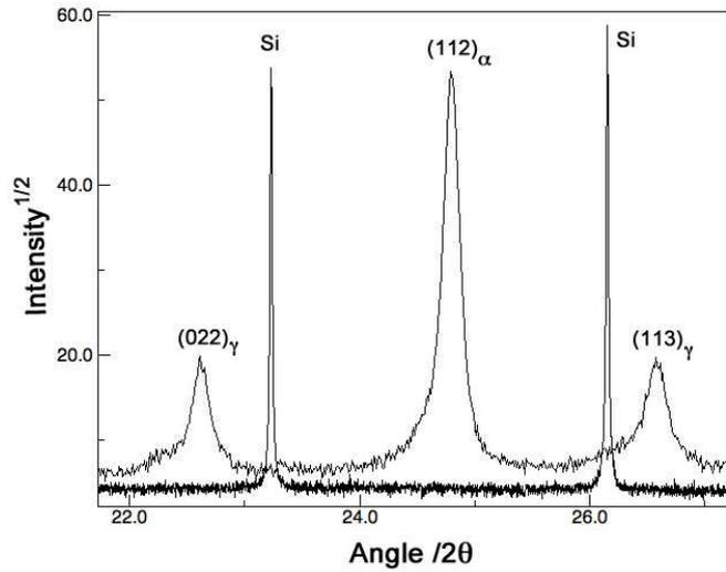
Figure 8. Superimposed peaks from the standard silicon sample.
