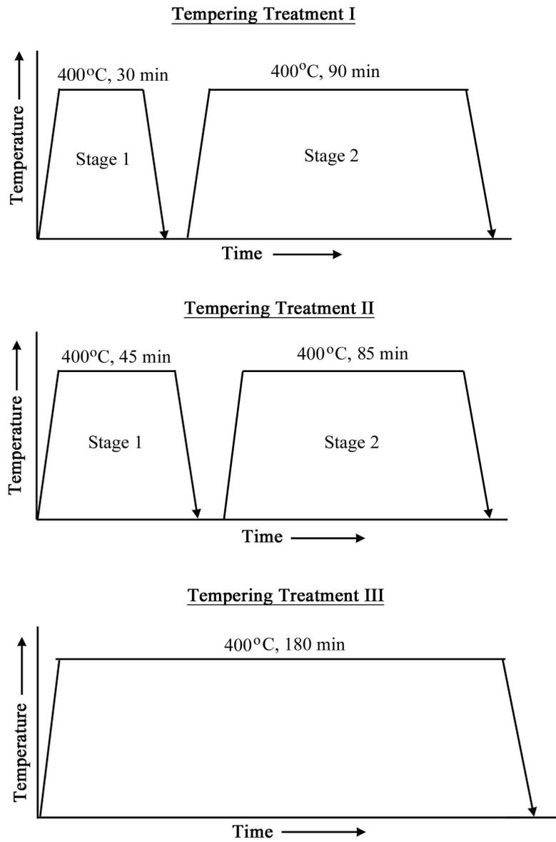
Figure 3. Tempering treatments carried out using synchrotron X-radiation. Arrows indicate the quench to room temperature.
