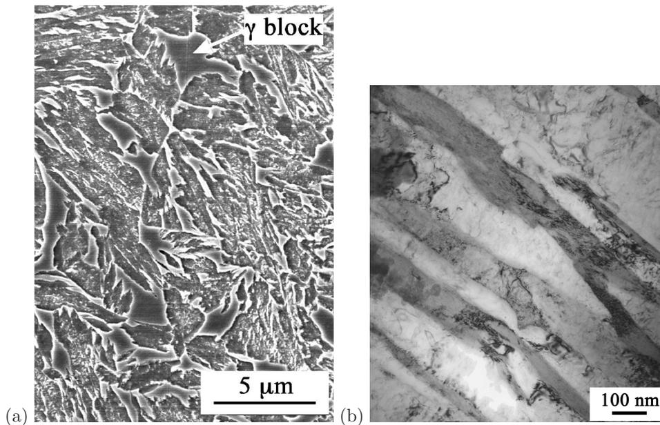
Figure 4. Sample isothermally transformed at 380°C. (a) Scanning electron micrograph illustrating the blocky regions of austenite. (b) Transmission electron micrograph showing bainitic ferrite with intervening films of retained austenite.
