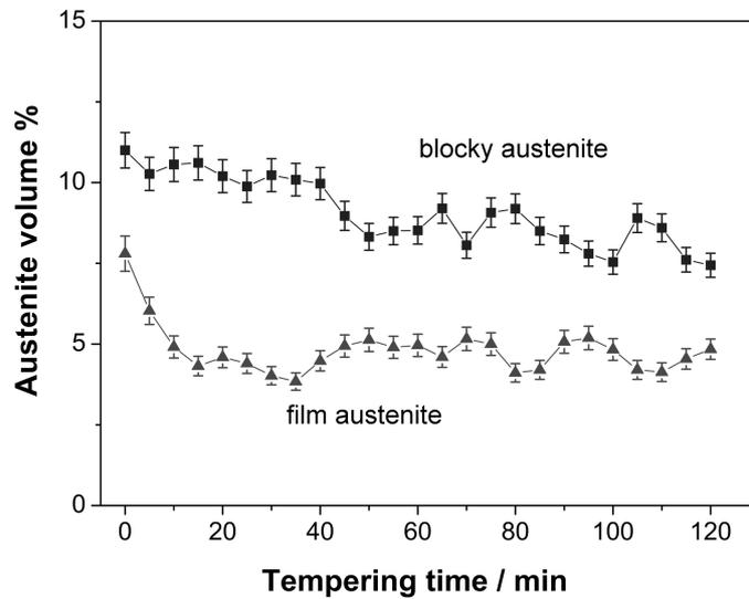
Figure 9. Change in amounts of blocky and film-type austenite at 400°C during tempering treatment-I.
