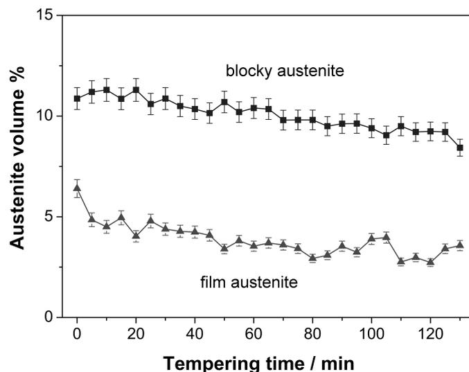
Figure 10. Change in amounts of austenite constituents at 400°C, measured during tempering treatment-II.
