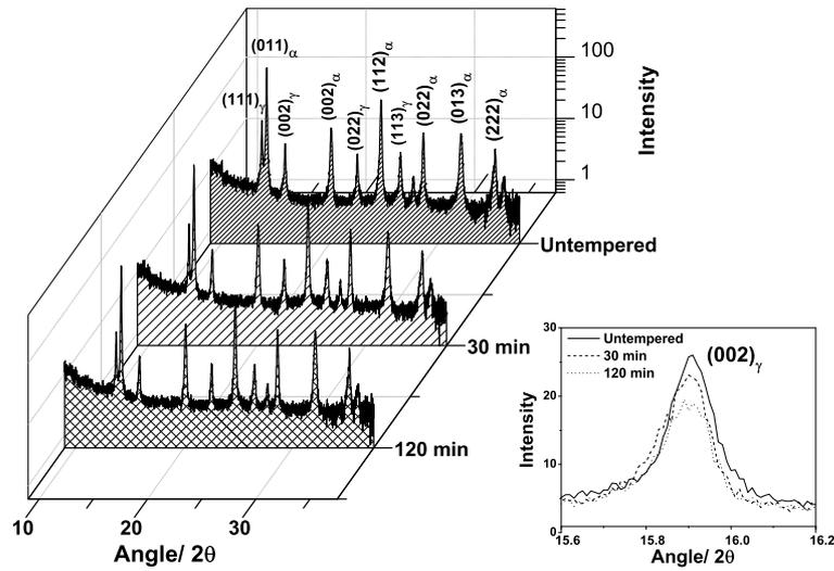
Figure 13. The plot showing synchrotron X-ray diffraction results after tempering treatment-I measured at room temperature.
