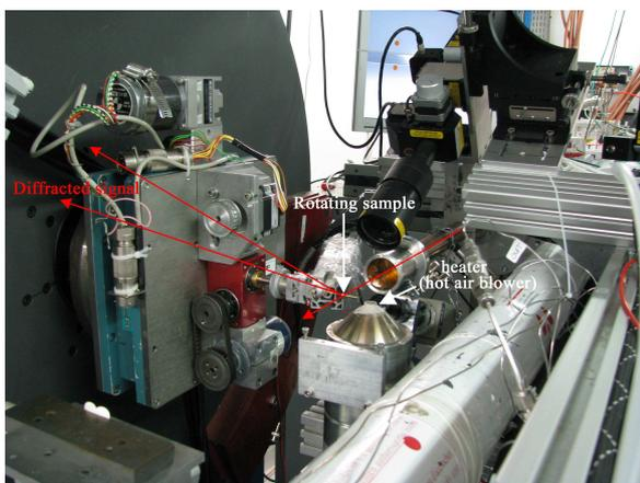
Figure 2. Sample assembly mounted at beam line with hot air blower positioned underneath.
