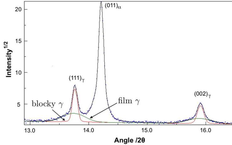
Figure 7. The figure shows deconvolution of two different types of austenite.
