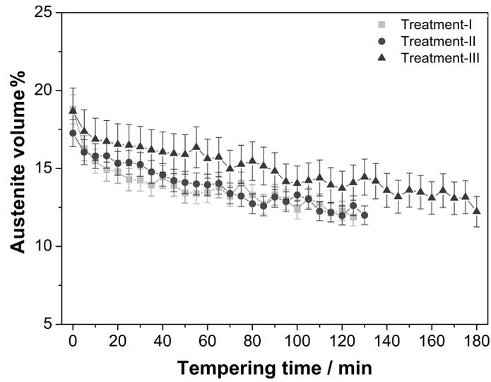
Figure 12. Measured volume% of retained austenite as a function of tempering time for three different tempering treatments.
