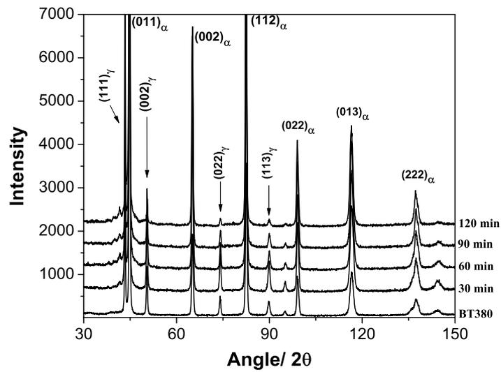
Figure 14. Results of low-energy X-ray diffraction. Isothermal transformation at 390°C (BT380) and followed by tempering at 400°C for different durations.
