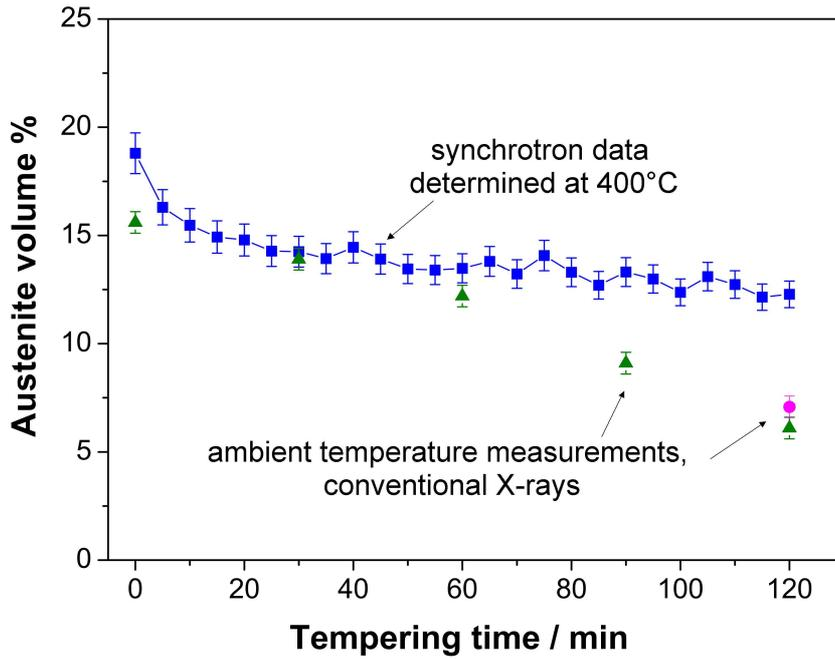
Figure 5. Retained austenite content as a function of time following tempering treatment-I.
