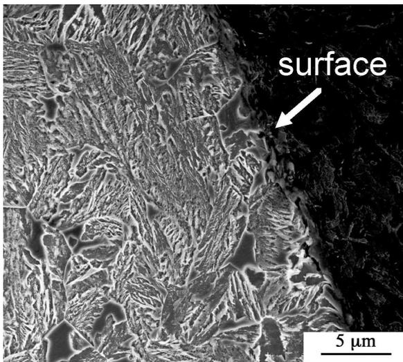
Figure 6. Scanning electron micrograph showing microstructure at the edge of the sample after tempering treatment-I.
