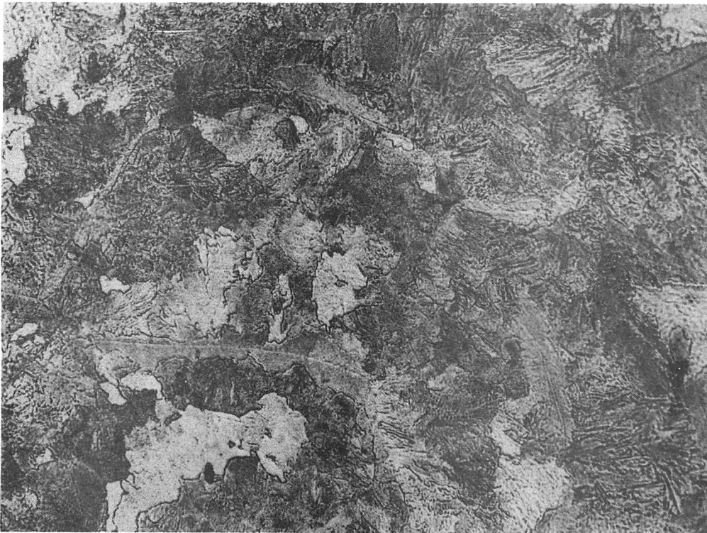
Fig. 24 Fe-4Mo-0.2C (Alloy B) isothermally transformed 72 hours at 650°C, X400.
