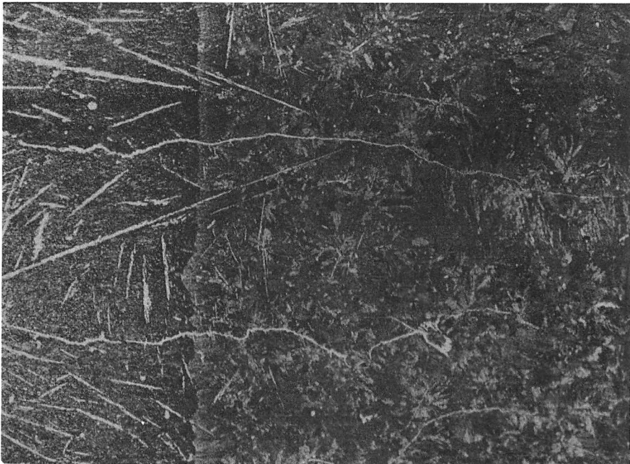
Fig. 45 Quenched interface in unidirectionally transformed Fe-1.2C (Alloy P9; V = 1.0 \times 10^{-4} cm/sec.), X4200.
