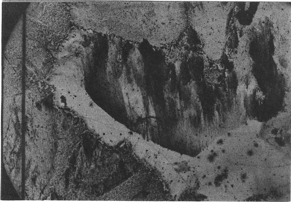
Fig. 6 Fe-1V-0.2C-1.5Mn (Alloy A3) isothermally transformed 15 min. at 650°C; carbon-extraction replica, X6000.
