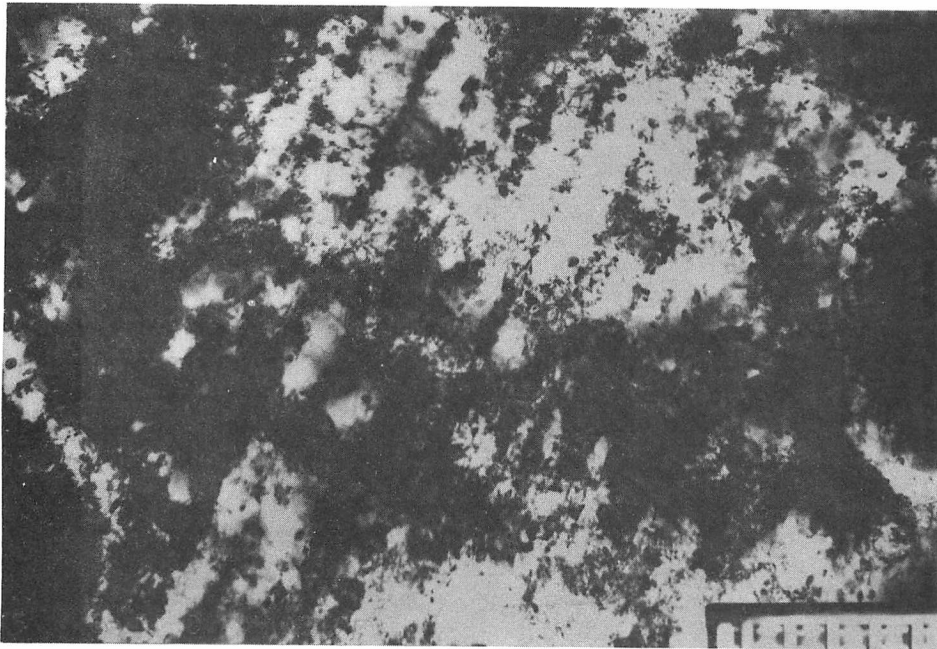
Fig. 14 Fe-1V-0.2C (Alloy A1) continuously cooled \sim 10\text{C}^\circ/\text{min} , and given \sim 80 percent rolling reduction; thin foil, X23,000.
