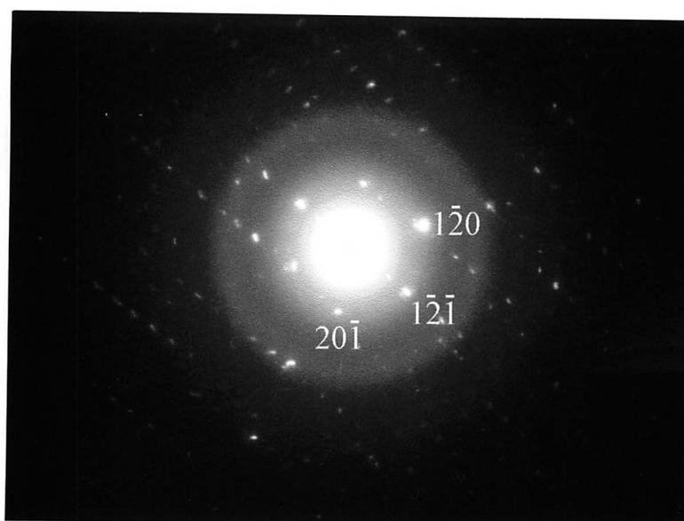
Figure 7.13 TEM micrograph of a cementite carbide in the carburised zone of a 2CrMo/ $\frac{1}{2}$ CrMoV dissimilar steel weld taken from service in the power plant. The zone axis of this diffraction pattern is  $[2\bar{1}4]$ .
