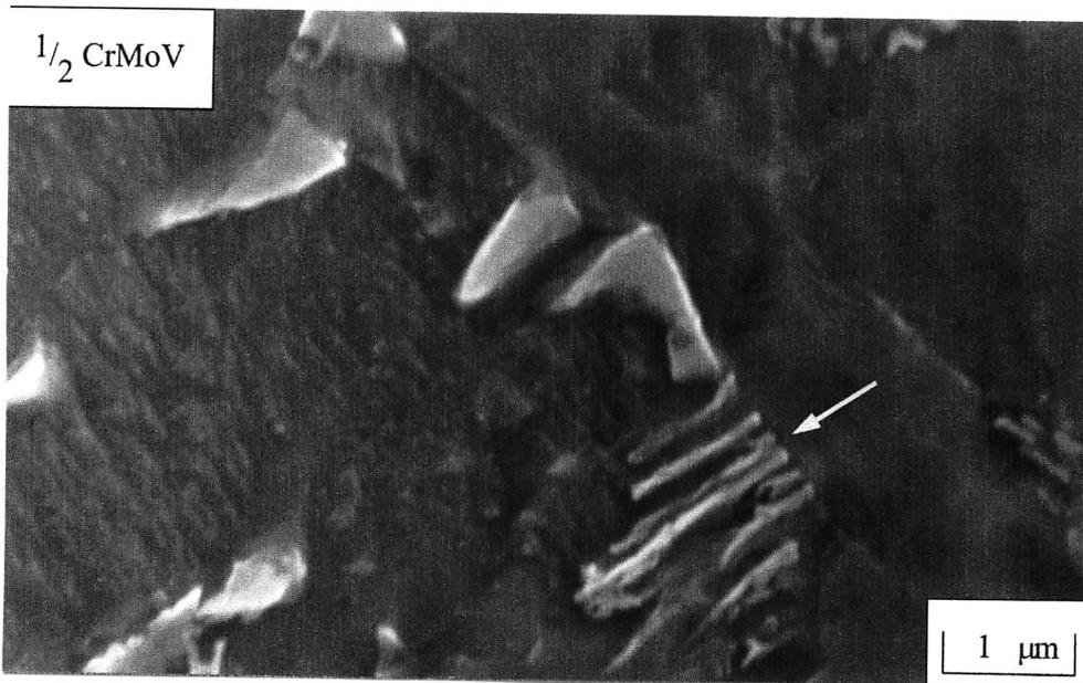
Figure 5.28 SEM micrograph of remnants of pearlite in the  $\frac{1}{2}$ CrMoV steel, immediately after bonding with a P91 steel.
