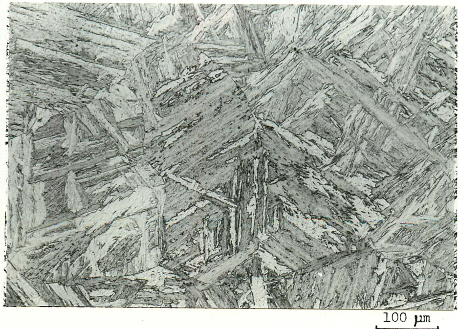
Figure 3.4: Martensite produced in Alloy 2 by iced-brine quench from 1200°C
