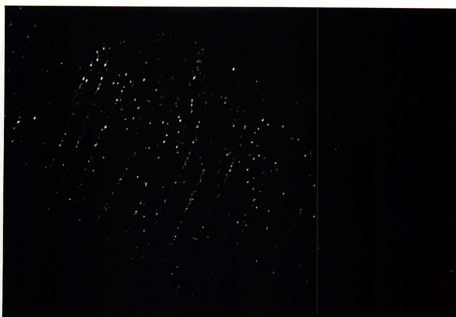
b) Precipitate centred dark field
