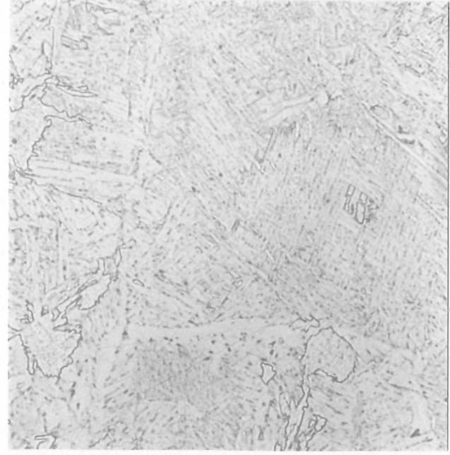
Figure 3.14: Bainitic structures 100 s 550°C, Alloy 1
