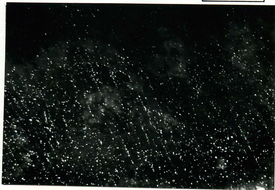
b) Precipitate centred dark field
