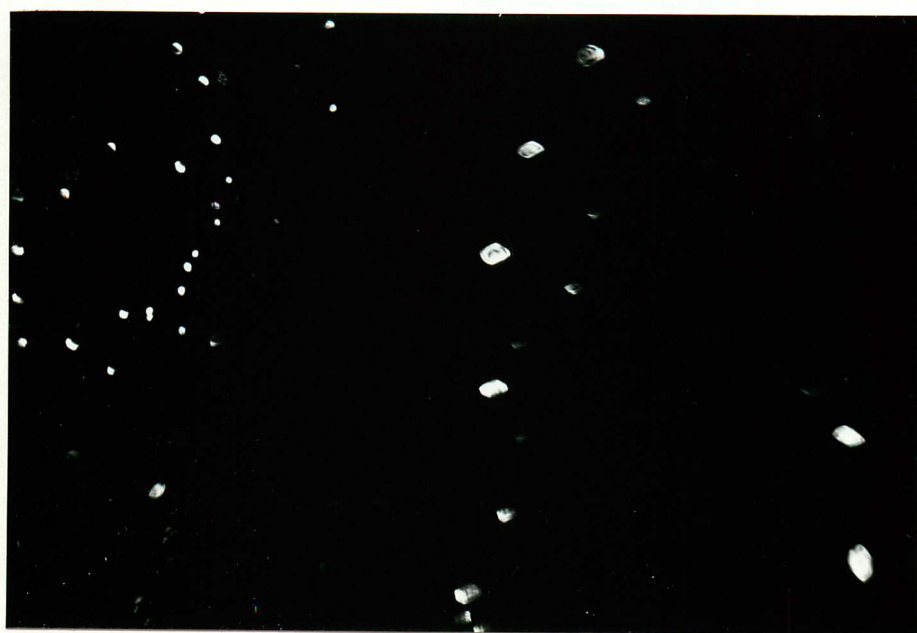
b) + 60 000 s 830°C precipitate centred dark field
