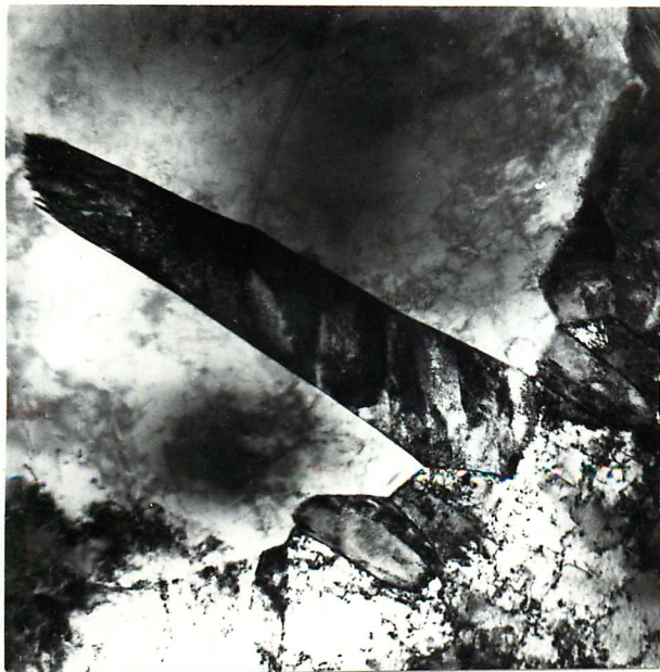
Fig. 3.12: a) Widmanstätten austenite sideplates at a ferrite grain boundary.
