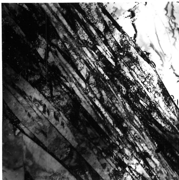
Fig. 6.6: Bright field - dark field pair of an austenite (now martensite) nodule containing retained austenite, imaged in dark field with an (002) diffraction spot. 15 mins 825 C.
