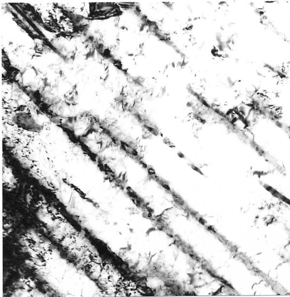
Fig. 5.7: Fibrous carbides dissolving in austenite leaving spheroidal carbides. A few seconds at 835°C.
