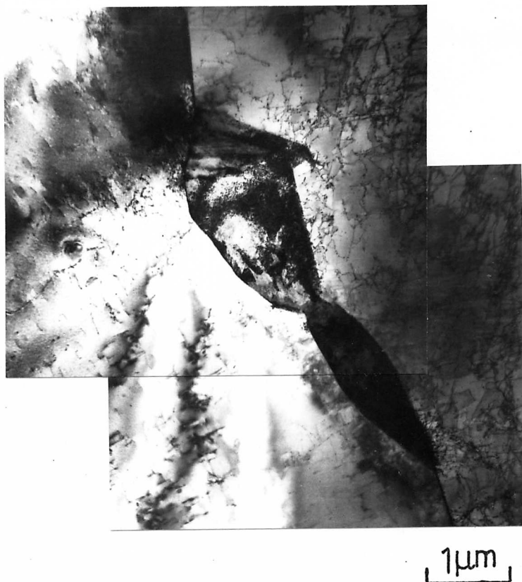
Fig 3.11: Austenite growing at a ferrite grain boundary showing partly faceted interfaces. Transformed 100s 750°C.
