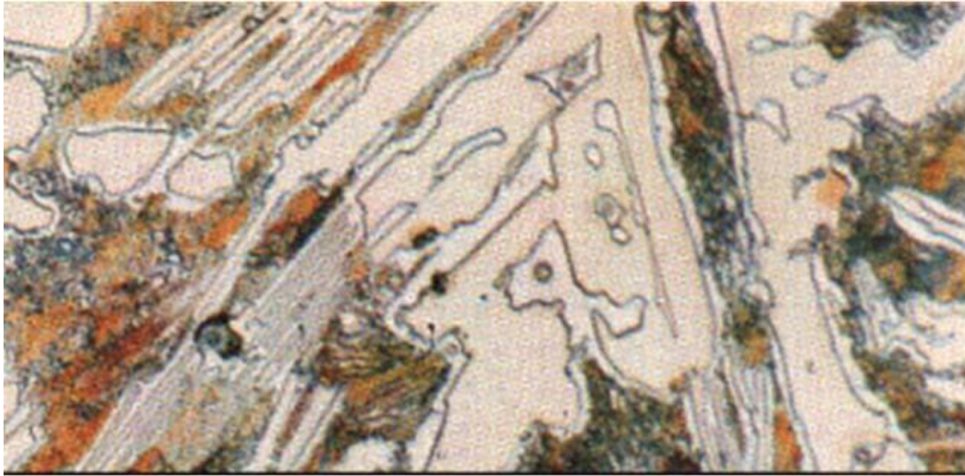
Fig. 12: High magnification view (400x) of the white cast iron specimen shown in Fig. 11, etched with 4% nital. After Mrs. Janina Radzikowska, Foundry Research Institute in Kraków, Poland
