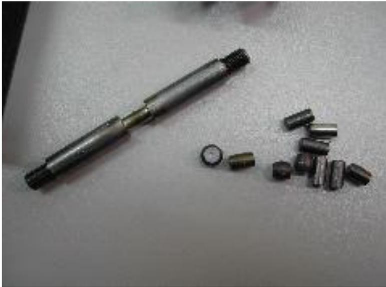
Fig . 3(a): Sample and fixtures for dilatometric measurements
