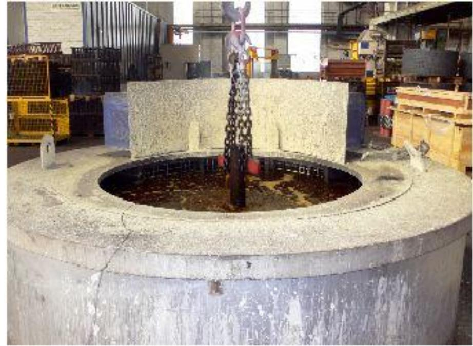
Fig. 2 : Bath II low-temperature salt-bath for isothermal treatment.
