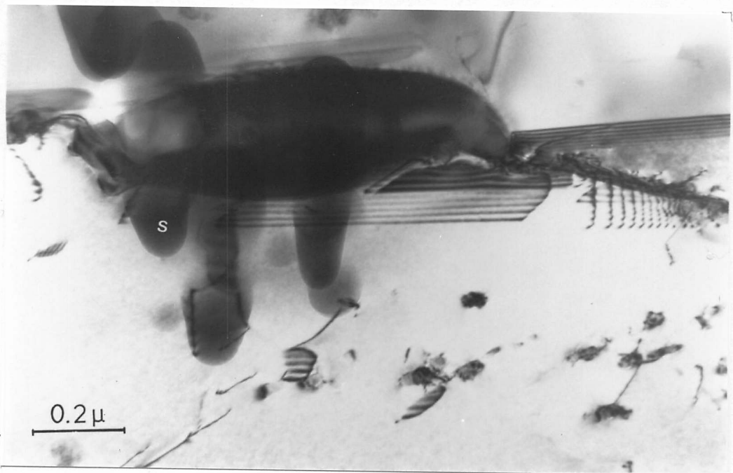
Fig 6.40 Isolated \sigma phase particle at grain boundary (contamination spots from EDS analysis are over the particle and matrix (S)). Aged at 900^\circ\text{C} for 100 hrs.
