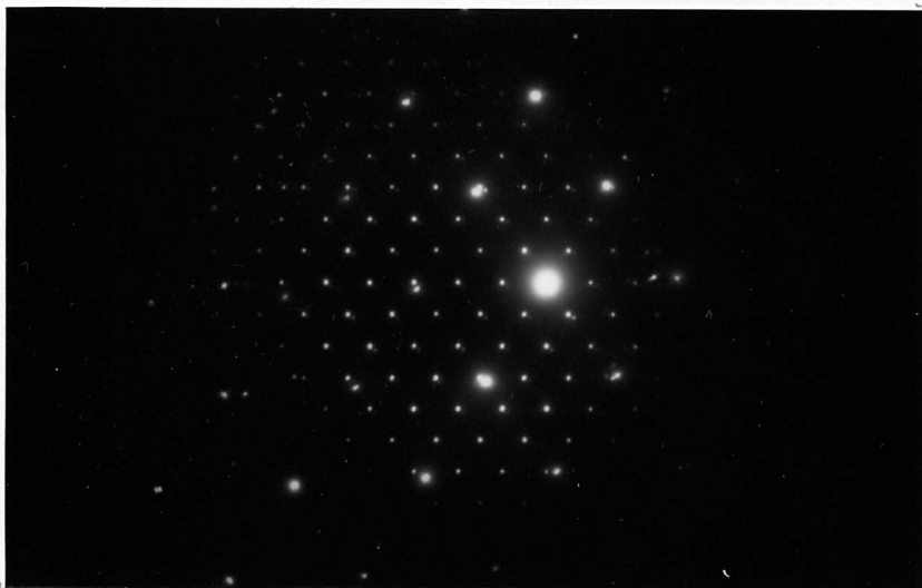
Fig 6.16 M_{23}C_6 precipitation at twin boundary. Aged at 700^{\circ}C for 1000 hrs. a) Bright field TEM image; b) Dark field image; c) SADP, zone axis: [011]_{\gamma} , [011]_{M_{23}C_6} .
