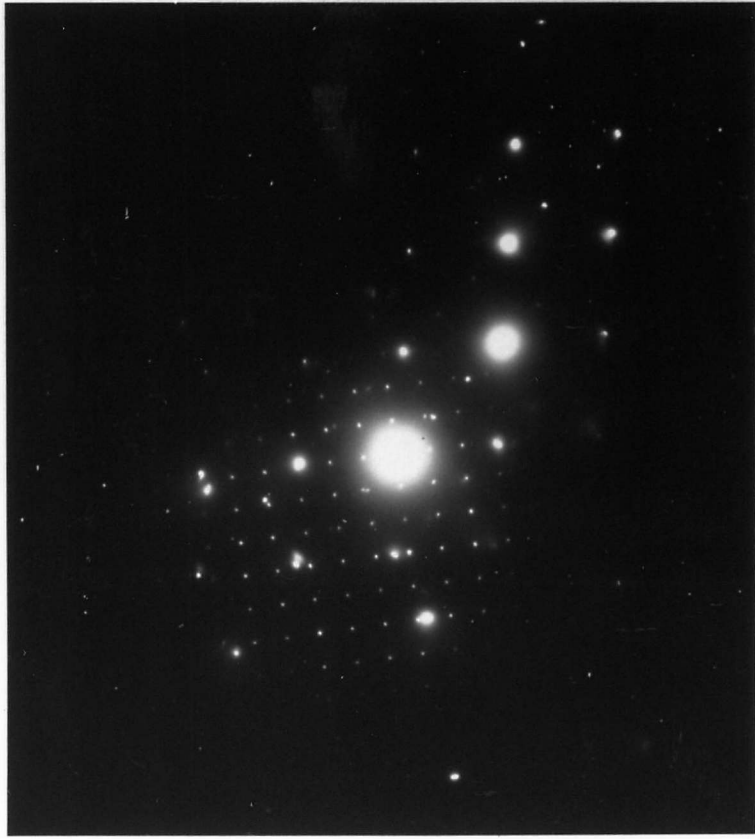
Fig. 6.32b Selected area electron diffraction of the precipitates, \text{Cr}_2\text{N} and X phase on grain boundary. Zone axis : [\bar{2}33]\text{Y} ; [001]\text{X} ; [01\bar{1}1]\text{Cr}_2\text{N} .
