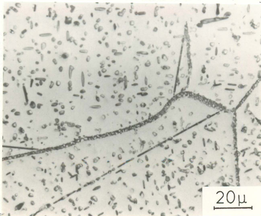
Fig 6.36 Optical micrograph showing matrix precipitation of faceted rod shape \chi phase. Aged at 800°C for 1000 hrs.
