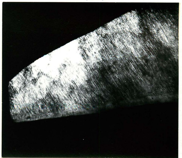
Fig. 3.15: Thin foil electron micrographs of Fe-IV-0.2C-1.5Ni directly transformed at 725°C for 30 secs. and quenched.
