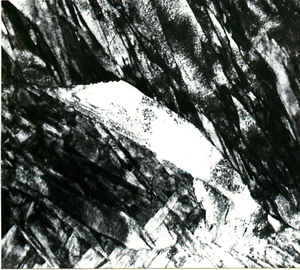
Fig. 3.16: Thin foil electron micrographs of Fe-IV-0.2C directly transformed at 675°C for 5 secs. and quenched.
