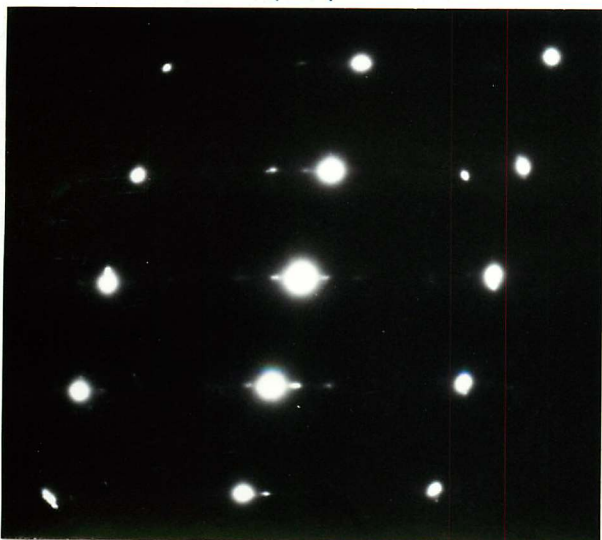
Fig. 2.5: Thin foil electron micrographs of double diffraction and twinning.
