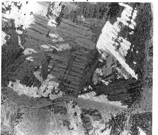
Fig. 4.4: Optical micrographs of the bainite structure.
