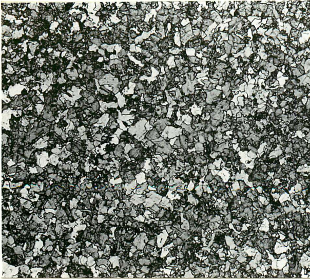
Fig. 5.1: Optical micrographs of the austenitised and retransformed structures.
