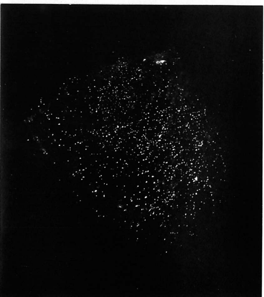
Fig. 4.12: Thin foil electron micrographs of the ferrite structure, transformed at 840°C for 15 secs. and iced brine quenched. (1) Bright field. (11) Centred dark field using a (020) austenite reflection. (111) Centred dark field using a (020) vanadium carbide reflection.
