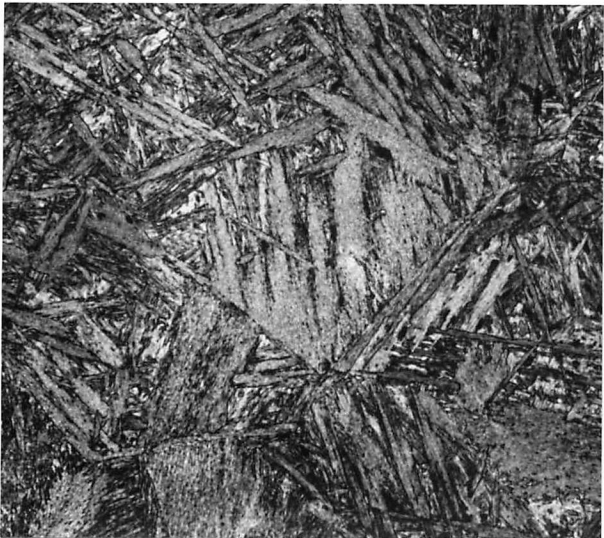
Fig. 4.4: Optical micrographs of the bainite structure.
