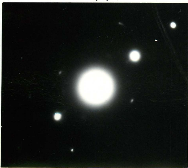
Fig. 4.14: Thin foil electron micrographs of the ferrite structure heated at 840^{\circ}\text{C} for 15 secs. and iced brine quenched. (i) Bright field. (ii) Centred dark field using a (020) austenite reflection. (iii) Diffraction pattern of the area shown in (i) (iv) Analysis of (iii). (v) Diffraction pattern of the matrix on the opposite side of the prior austenite boundary. (vi) Analysis of (v).
