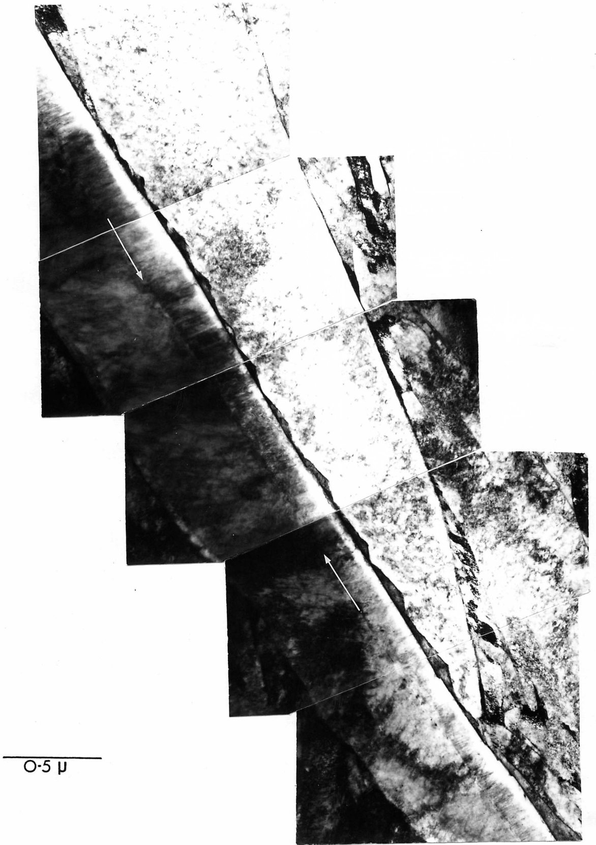
Fig. 3.13b: Composite thin foil electron micrograph of Fe-IV-0.2C-1.5Mn directly transformed at 725°C for 30 secs. and quenched.
