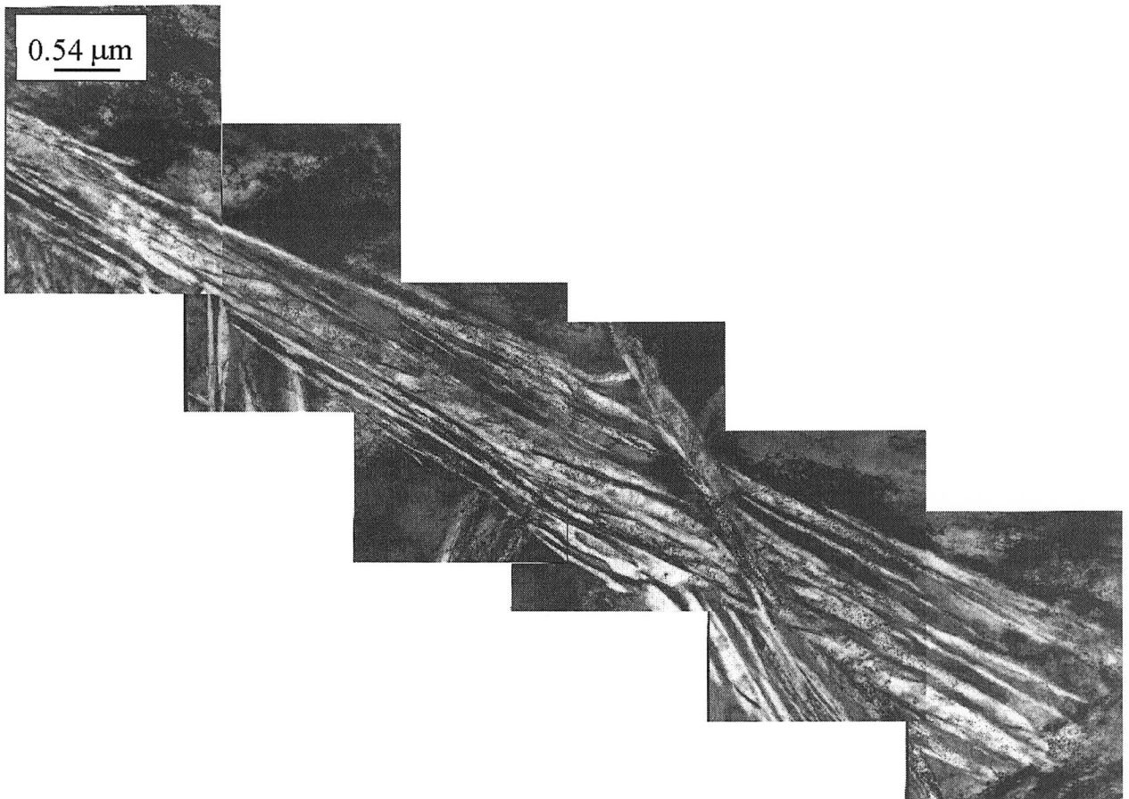
Fig. 1.8: Montage of transmission electron micrographs showing the structure of a bainite sheaf in a high-carbon high-silicon steel transformed at 200^{\circ}\text{C} for 15 days [Courtesy of Garcia Mateo and Bhadeshia].
