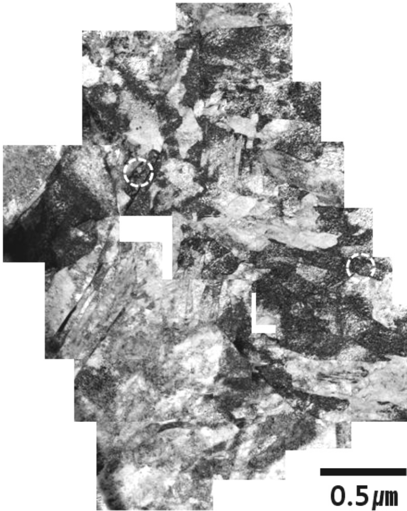
Figure 5.11: Transmission electron micrograph of a region extracted using focused ion beam machining from bainite identified using scanning electron microscopy, in the heterogeneous sample. The circled areas were then subjected to microanalysis.
