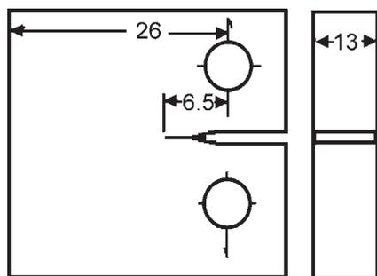
3 Dimensions of compact tension sample in mm, with diameter of holes being quarter of sample thickness
