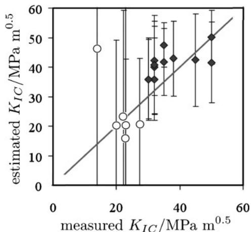
4 Comparison of measured fracture toughness of superbainite both in isothermally transformed (solid points) and tempered (unfilled circles) conditions, against model estimates: error bars represent  $\pm 1\sigma$  modelling uncertainty and it is emphasised that some of values plotted are  $K_Q$  data as explained in Table 3
