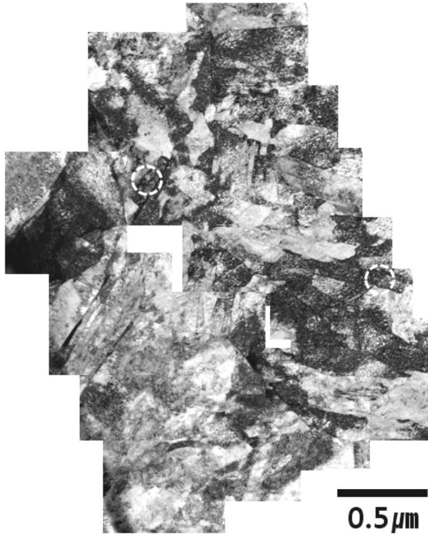
Figure 10: Transmission electron micrograph of a region extracted using focused ion beam machining from bainite identified using scanning electron microscopy, in the heterogeneous sample. The circled areas were then subjected to microanalysis.
