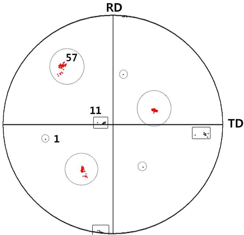
Fig. 4.  $\{001\}$  pole figure showing the orientations of 69 separate coalesced bainite regions, where RD represents the tensile direction. The number of observations for each orientation is indicated by the figures 1, 11 and 57.
