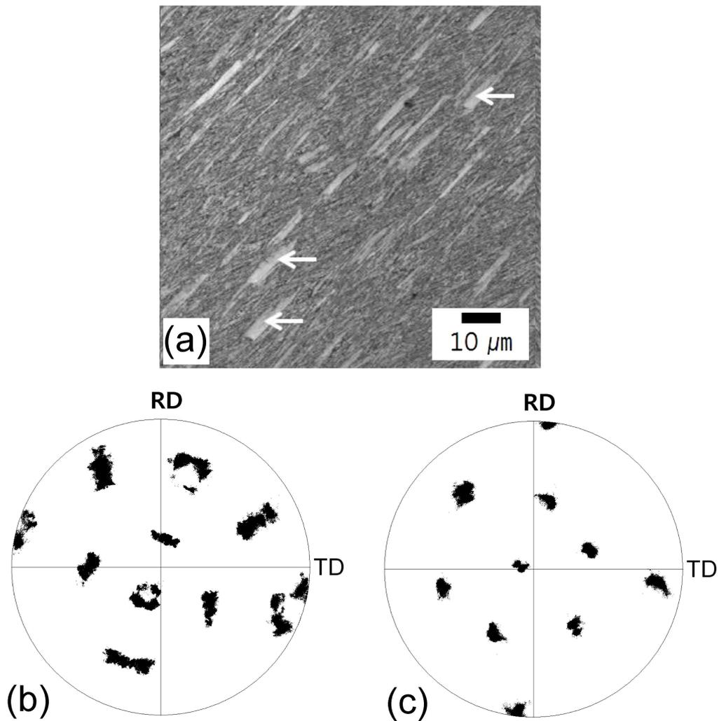
Fig. 3. (a) Image quality map of stressed sample, the orientation of the stress is identical to Fig. 2b. (b)  $\{001\}$  pole figure from a single grain of unstressed austenite, showing intensity from a large number of variants. (c) Corresponding pole figure from stressed austenite, with the tensile axis along 'RD'
