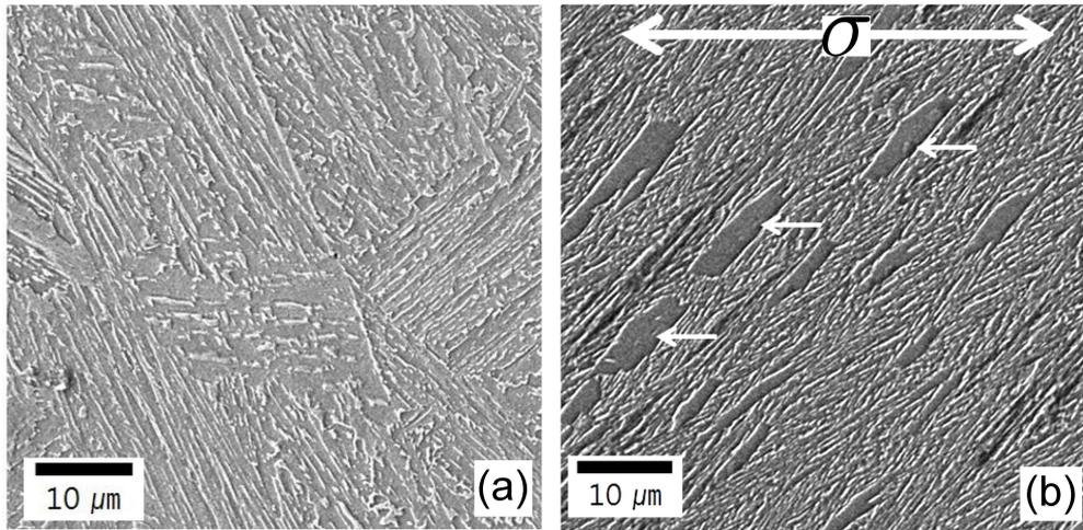
Fig. 2. (a) Stress-free transformation. (b) Transformation under the influence of a tensile stress  $\sigma$  along the orientation indicated. The short arrows show the coalesced bainite.
