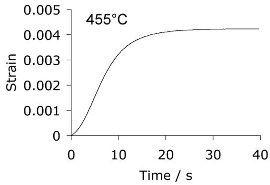
Fig. 1. Dilatometer data for isothermal transformation to bainite at the temperature indicated.
