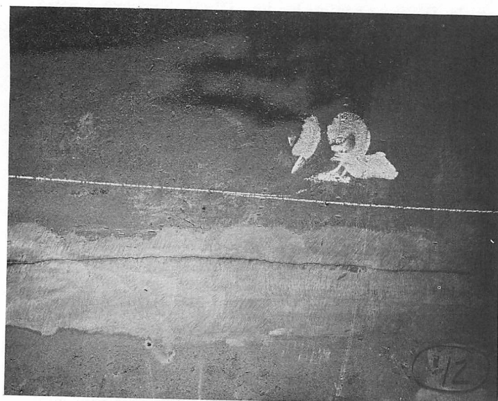
a. Typical brittle appearance of crack on inside surface.
