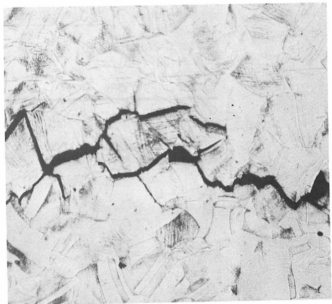
FIGURE 8—Hydrogen embrittlement of Hastelloy Alloy C-276 in 5% NaCl, 0.5% acetic acid saturated with H_2S . C-ring specimen galvanically coupled to steel.
