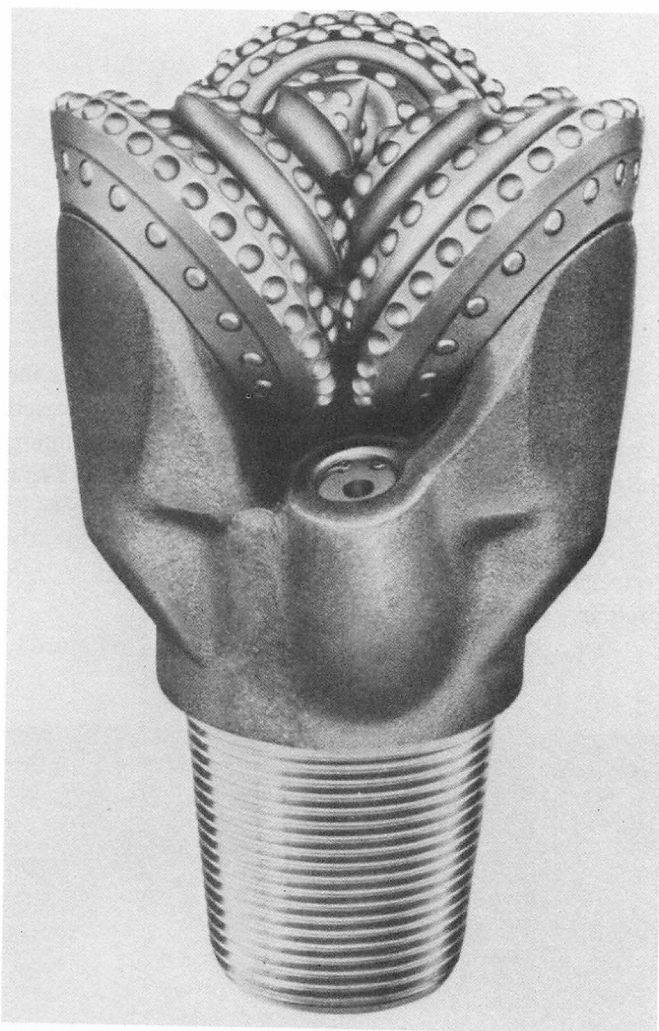
FIGURE 4—Tungsten carbide tooth, hard formation bit manufactured about 1960. Note the cemented carbide jet nozzles introduced in 1953. [Gauge diameter 220 mm (8 3 / 4 in.)]
