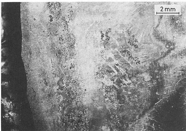
a. Numerous pits in the base material.
