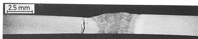
a. Combination 25 Cr-25 Ni-2.5 Mo/AISI Type 321; many stress corrosion cracks in T 321, no cracks in 25 Cr-25 Ni-2.5 Mo.
