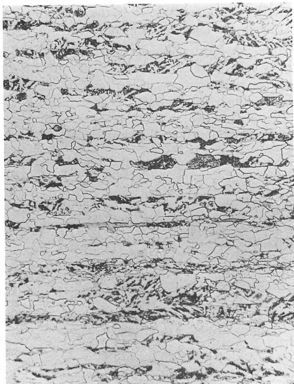
FIGURE 5—Microstructure of control rolled Mn-Mo-Nb steel. 2% Nital etch.
