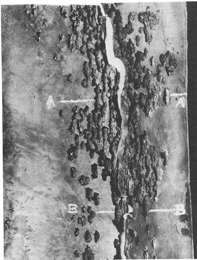
FIGURE 3—Corrosion of steel in sour field environment.
