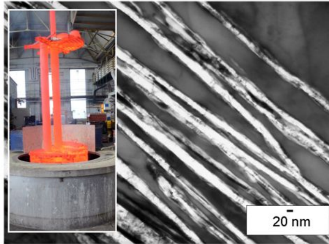
Fig. 3. Extremely thin plates of bainitic ferrite embedded in a matrix of austenite. Inset: large scale processing of new steel.
