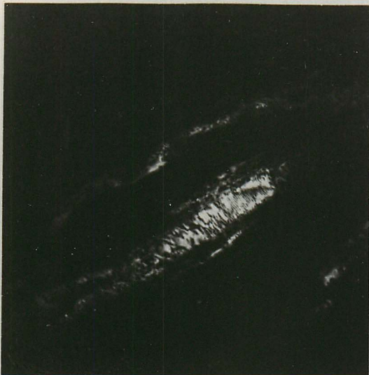
Fig. (3:17e) TEM of T/S of A/R + LTHT "B" patented wire ( \alpha CDF) X200,000
