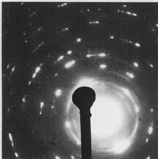
Fig. (3:10c) TEM of L/S of A/R patented wire (SADP for (3:10d))
