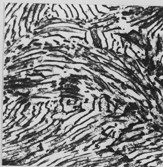
Fig. (3:13d) TEM of T/S of A/R + LTHT "A" patented wire (BF) X50,000
