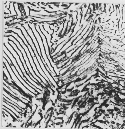
Fig. (3:13b) TEM of T/S of A/R + LTHT "A" patented wire (BF) X60,000
