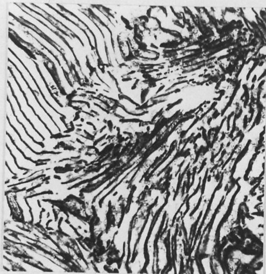
Fig. (3:13a) TEM of T/S of A/R + LTHT "A" patented wire (BF) X60,000
