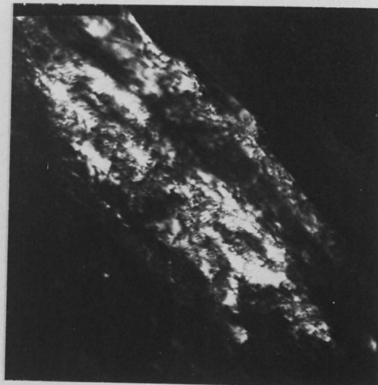
Fig. (3:14b) TEM of L/S of A/R + LTHT "A" patented wire (α CDF)
