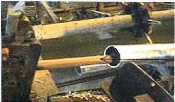
Novel tube inner wiping system to remove excess zinc
