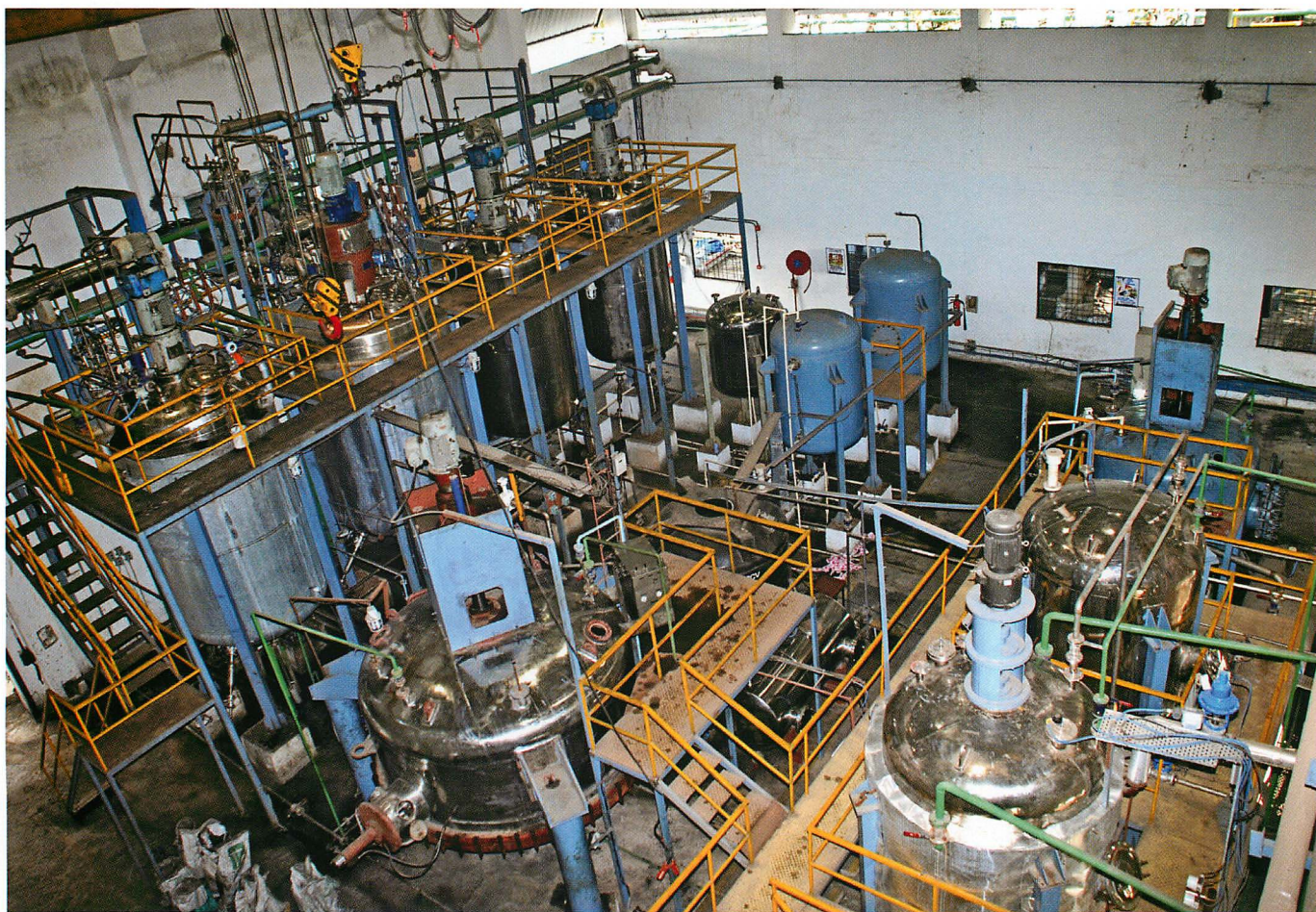
Semicontinuous pilot plant for chemical beneficiation of coal (2011)
