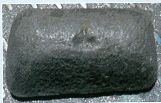
Trapezoidal shaped pig iron ingot
