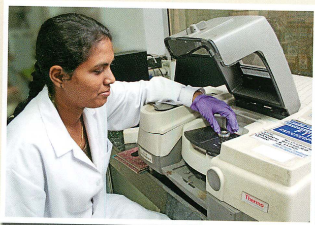
Fourier Transform Infrared Spectroscopy in the Advanced Corrosion Laboratory
