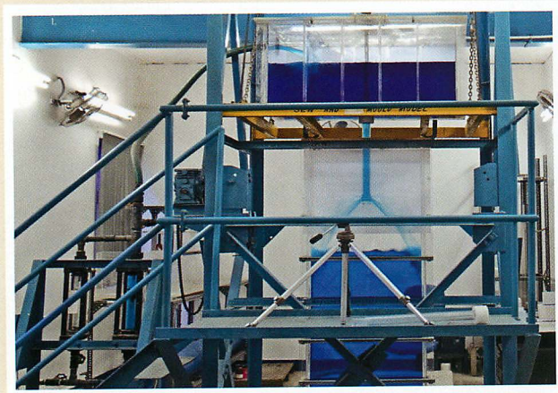
Scaled down water model of the Slab Caster facility at Tata Steel
