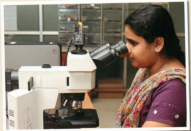
Carl Zeiss Optical Microscope equipped with high resolution camera
