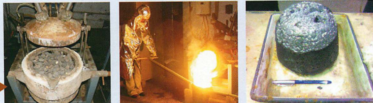
Sponge chrome process trials in industrial tunnel kiln furnace
