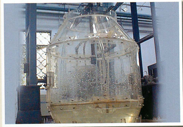
Scaled down water model of the LD Vessel
