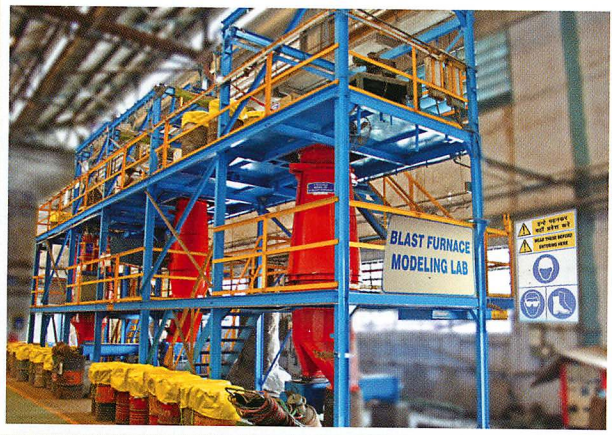
1:10 scaled down models of Tata Steel blast furnaces equipped with bell less charging system
