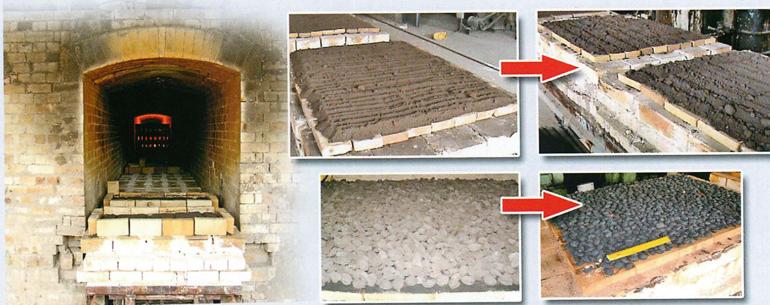
Sponge chrome process trials in industrial tunnel kiln furnace
