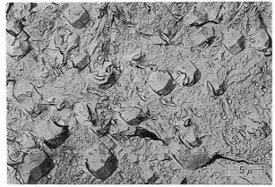
Photo. 20. An example of etch pits showing (001) a formed on a large brittle fracture facet of tempered upper bainite in steel 2.  $1300^{\circ}\text{C} \times 30 \text{ min } 470^{\circ}\text{C}$  Q+600°C×1hr.
