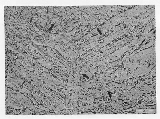
Photo. 6. Electron micrograph for steel D tempered at 450°C showing grain-boundary precipitation of carbides (arrows).
