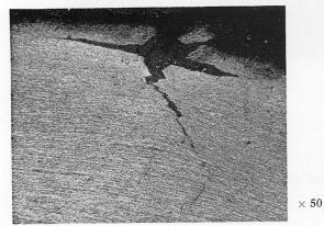
Photo. 7. Cross section of bend-test specimen of hot-stripmill-rolled low-carbon bainitic steel. Nital etch.
