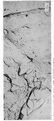
a) Intergranular fracture with dimpled rupture.
