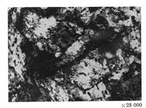
Photo. 2. Thin-foil micrograph of 1% Cr steel isoformed at  $550\,^{\circ}\text{C}.$
