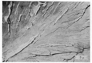
Photo. 19. Fracture surface of tempered upper bainite in steel 2.  $1300^{\circ}\text{C} \times 30 \text{ min } 470^{\circ}\text{C Q} + 600^{\circ}\text{C} \times 1\text{hr.}$
