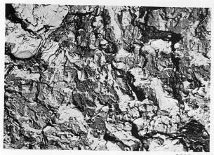
Photo. 12. Typical quasi-cleavage fracture.  $\times 3000 \times 4/5$  Charpy fracture at room temperature.)
