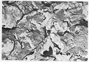
$\times 3000 \times 4/5$  Photo. 17. Carbides separated from matrix at the carbidematrix interface. (Sample F, static bend fracture.)
