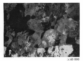
Photo. 3. Thin-foil micrograph of martensitic carbon-manganese steel deformed at 600°C.
