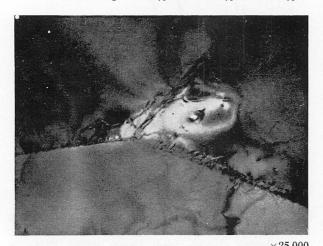
Photo. 2. Transmission electron micrograph of ferritic steel containing 16.74% Cr, 0.002% C, 0.022% N.
