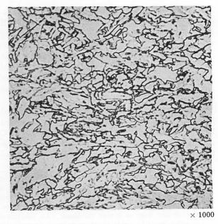
Photo. 10. Representative microstructure of manganese-molybdenum-niobium X-65 linepipe steel.
