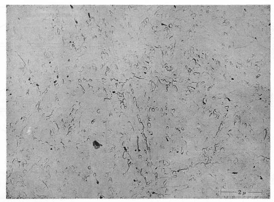
Photo. 9. Electron micrograph of chromium-molybdenum-vanadium steel tempered at 600°C after isothermal transformation at 325°C showing spheroidized carbides at prior austenitic grain boundary.
