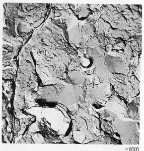
Photo. 15. An example of carbide-cleavage on the fracture surface.
