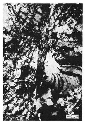
Fig. 2. Transmission electron micrograph of the area just below the fracture surface. A spheroidized 0.2% C steel bar was fractured by tension. The fracture surface was electroplated with iron and subjected to thin foil preparation. The fracture surface is from the upper right to the lower left. Electroplated iron is right side of fracture surface.
