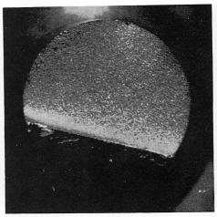
Photo. 10. Fracture surface of a fatigue-test specimen. (Sample B: 95 kg/mm², N=86 800.)
