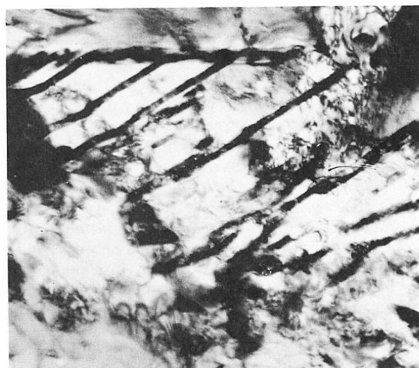
FIGURE 9. High carbon upper bainite produced by enrichment of austenite in carbon in a low carbon steel; thin foil electron micrograph, 60,000 X
