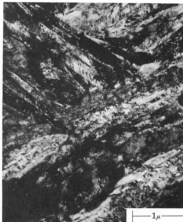
FIGURE 17. Aggregate lower bainite in S steel transformed at 275 C (525 F) for 17 hr. 21,200 X
