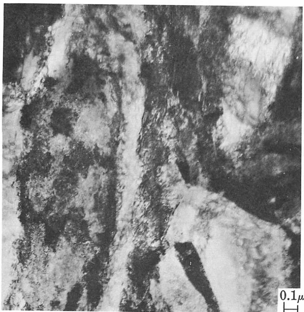
FIGURE 18. High dislocation content and inhomogeneous defect density in ferrite after thermomechanical treatment of manganese-molybdenum-boron steel VII by 30% deformation between 650 and 550 C (1200 and 1020 F) and cooling at 80 C/min (145 F/min). Thin-foil electron micrograph
