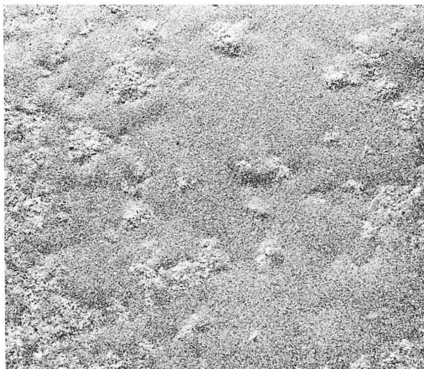
FIGURE C. "Fine-grained" 8620 steel thermally etched 11 hours at 925 C (1700 F). 500 X
