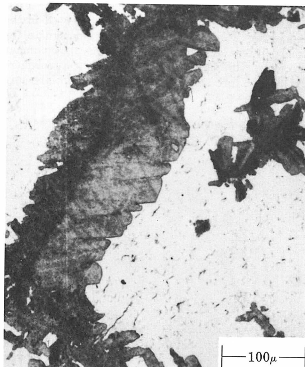
FIGURE 12. Light micrograph of columnar bainite formed at 290 C (550 F) and 24 kbar
