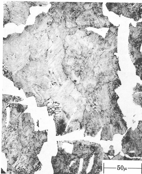
FIGURE 6. Light micrograph of 0.44% C steel as normalized at one atmosphere
