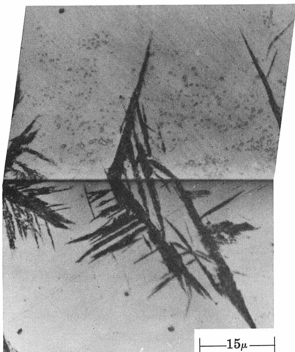
FIGURE A. Two-surface composite micrograph of lower bainite in an Fe-7.9 Cr-1.1C alloy
