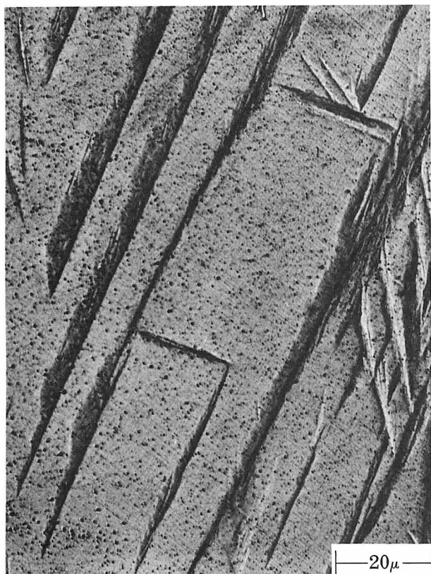
FIGURE B. Lower bainite plates in surface relief; oblique illumination
