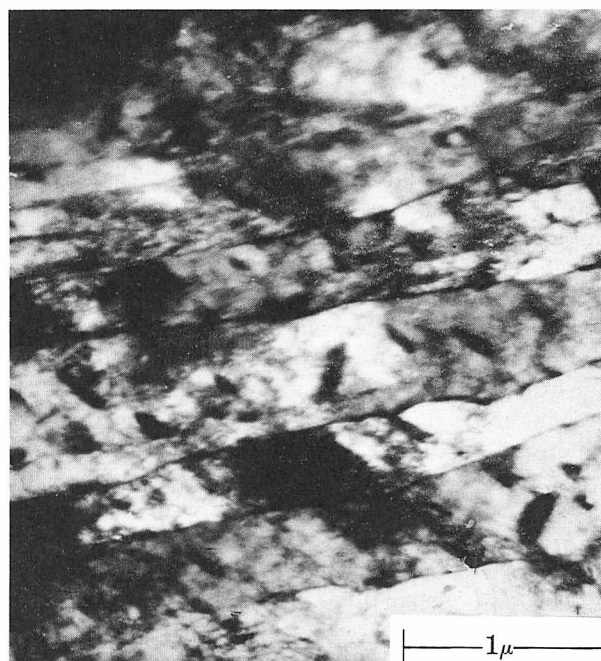
FIGURE 19. Upper bainite containing internal carbides in 1040 steel transformed at 435 C (815 F) for ten minutes. 27,700 X
