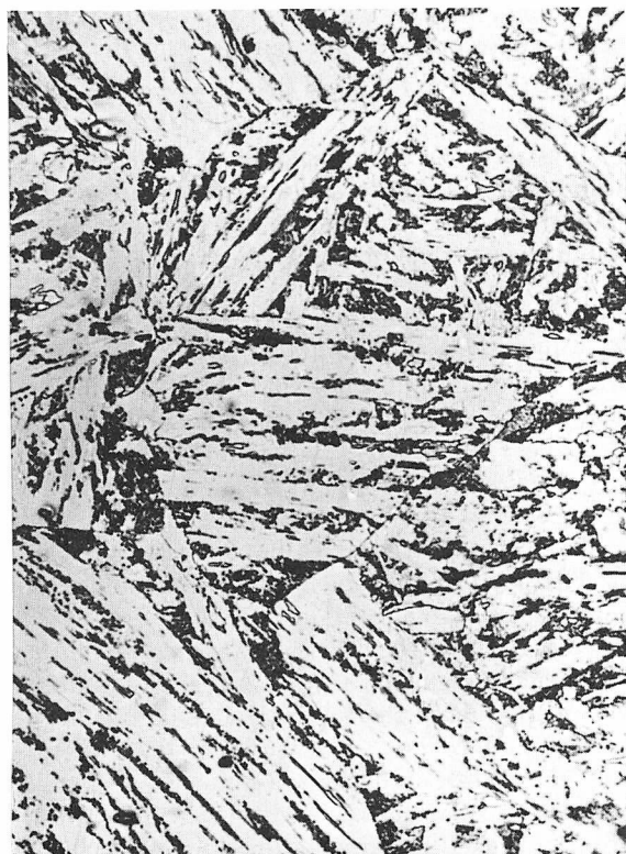
FIGURE 17. Austenitic-martensitic areas replaced by ferrite-carbide aggregates in manganese-molybdenum-boron steel VII thermomechanically treated by 30% deformation between 800 and 700 C (1470 and 1290 F) and cooled at 80 C/min (145 F/min). Optical (500 X) and thin-foil electron micrograph.
