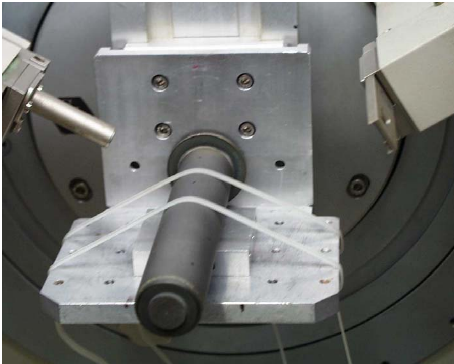
Figure 8.1 Photograph showing residual stress measurement in the hoop direction of a shot peened steel bar. Note the use of cable ties to hold the sample in place, along with a U or V shaped holder. (Courtesy of QinetiQ Ltd)
